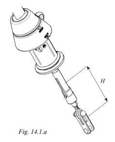
The rigging screw has a stop at the maximum position to which it can be unscrewed. Do not overload this stop by trying to unscrew the rigging screw further. The values given in the table below for adjustment must not be exceeded!
