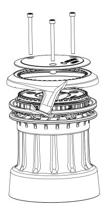
Beware of any inteference between the load and non load end of the line while operating the winch. Adjustment of the self-tailing arm may be needed to avoid any interference.
