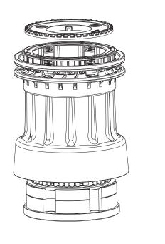
Remove the roller-bearing and the washer. Follow this by unscrewing the five (5) screws locking the centre hub to the base. Depending on the version of the winch, this is done using a hexalobular key size T30 or a 5mm Allen-key.
