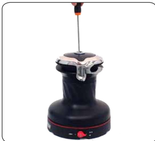
2. Unscrew the central screw ( \approx 2\text{Nm}/18\text{ in-lb} )
