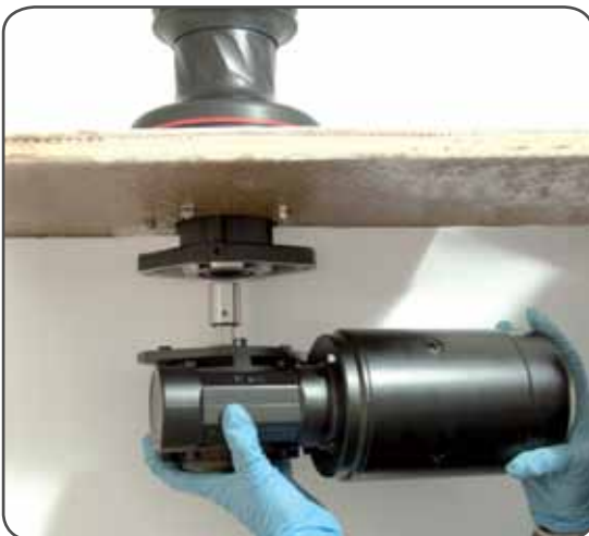
3. Position the reduction gear and motor
