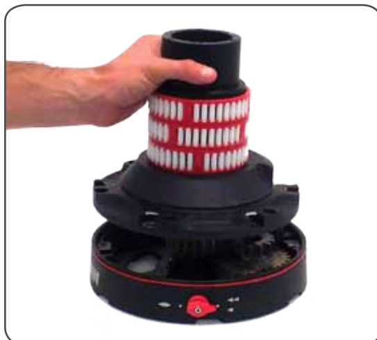
9. Remove the assy drum support n°13
