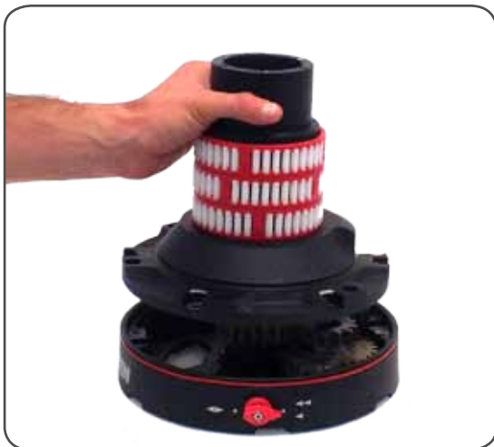
9. Remove the assy drum support n°13
