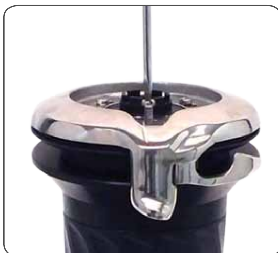
4. Unscrew the three screws n°41 ( \approx 4\text{Nm}/35\text{ in-lb} )
