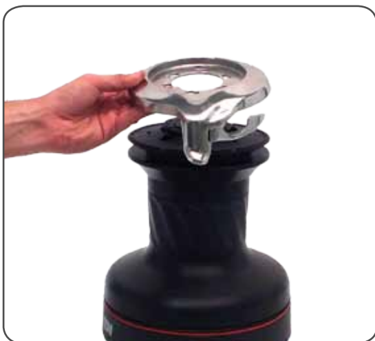
5. Remove the stripper arm n°44 by rotating and lifting it.
