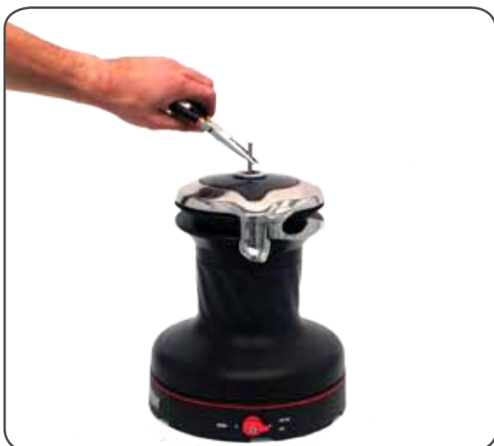
1. Pull out the disconnect rod n°21
