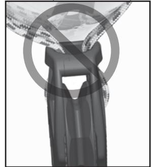
If you have access to end of boom, twist each lap. Secure using double fisherman's knot or other secure knot. See "Lashing to Bail Using Harken Supplied Line" below.
