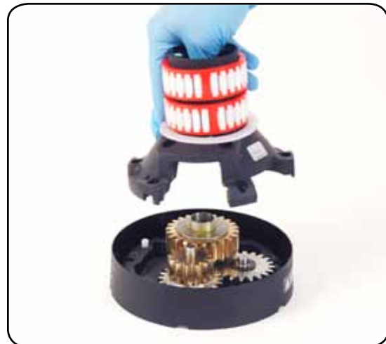
9. Remove the assy housing n° 15 Important: washer n° 12 may remain inside the drum support!
