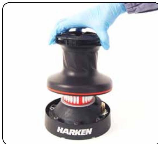
6. Lift off the drum n°22
