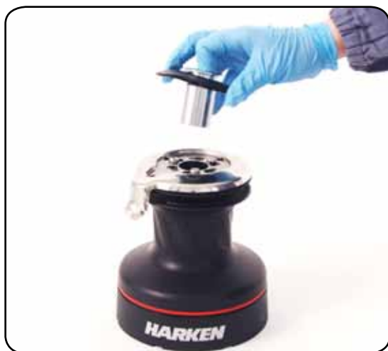
3. Slide off the assy socket n°28 and the cover n°29.
