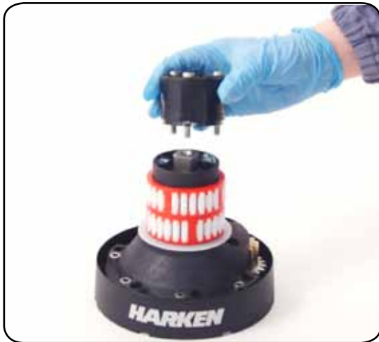
6. Completely unscrew the three screws n° 27 and remove the stripper arm support n° 21
