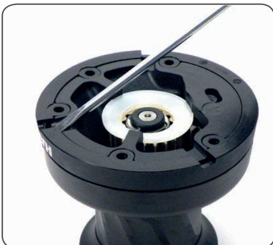
1. Remove the skirt n°2 with the help of the screwdriver placed as shown by the symbol
