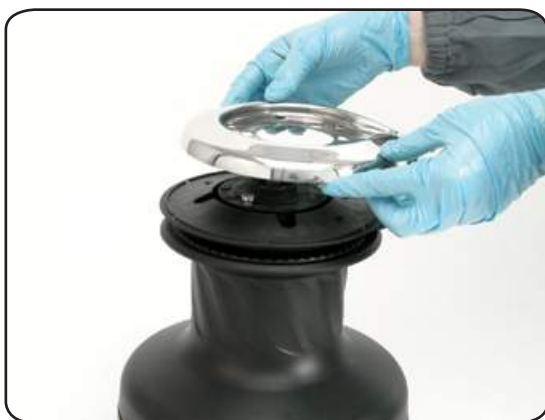
5. Remove the self-tailing arm n°27 by rotating and lifting it.
