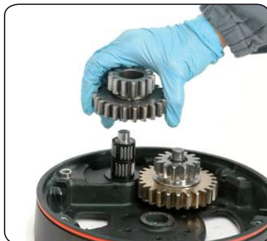
14. Remove the idler and pinion n°14
