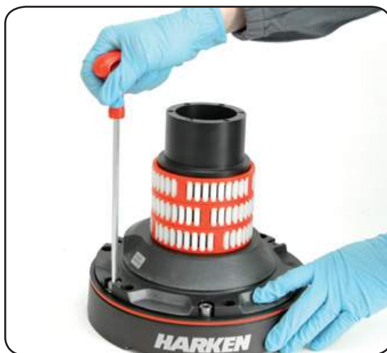
10. Unscrew the 6 hex screws n° 17 ( 20Nm/177 in-lb)
