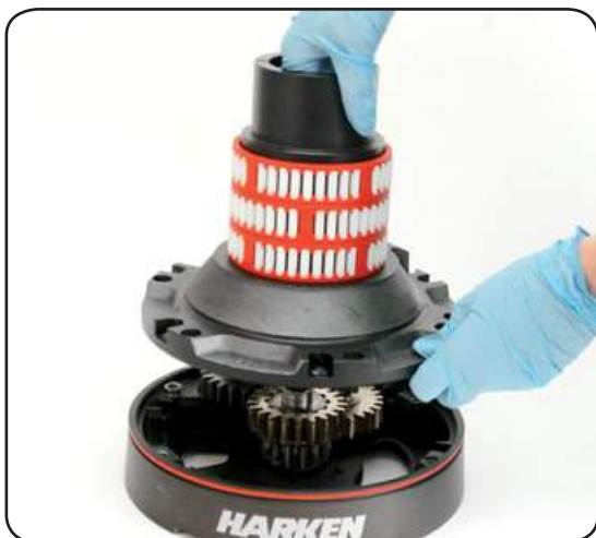
11. Remove the drum support n° 16
