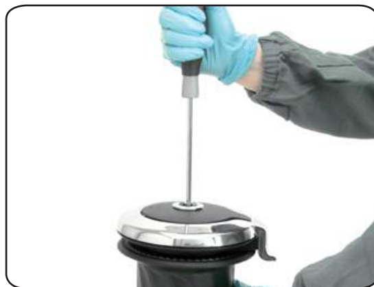
2. Unscrew the central screw ( \approx 2\text{Nm}/18\text{ in-lb} )
