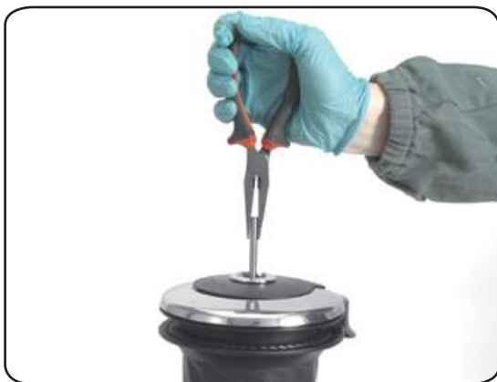
1. Pull out the disconnect rod n°31
