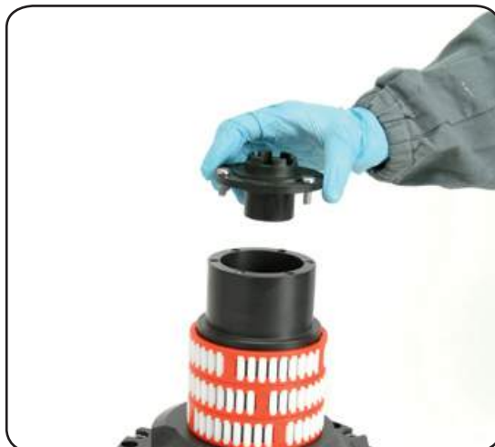
8. Remove the stripper arm housing n° 21
