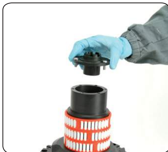
8. Remove the stripper arm housing n° 21
