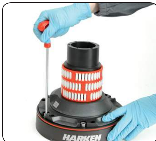
10. Unscrew the 6 hex screws n° 17 ( 20Nm/177 in-lb)
