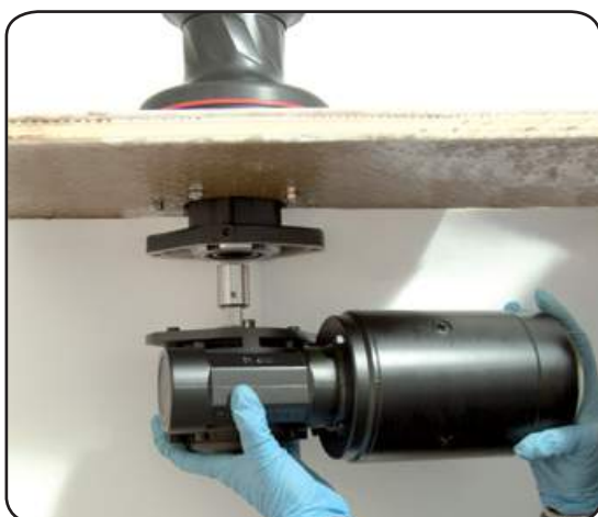
3. Position the reduction gear and motor
