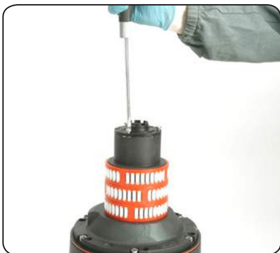
7. Completely unscrew the three screws n° 28
