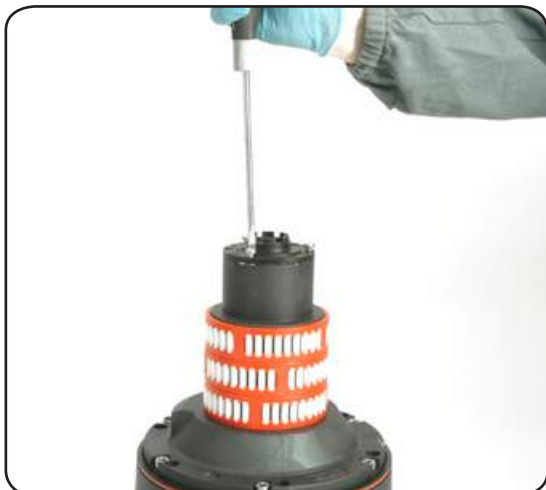
7. Completely unscrew the three screws n° 28
