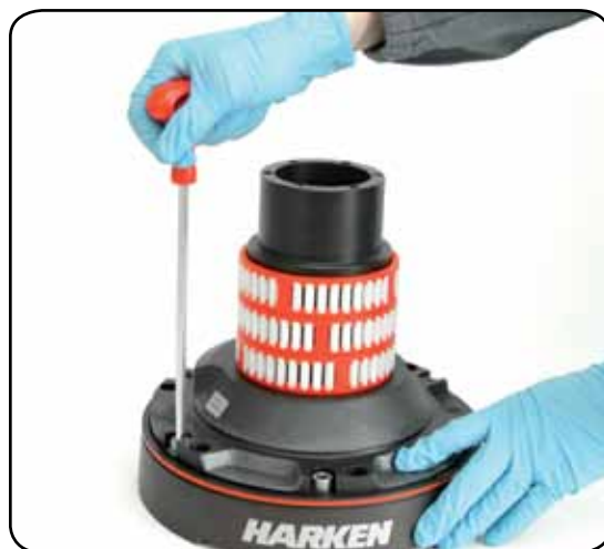
10. Unscrew the 6 hex screws n° 17 ( 20Nm/177 in-lb)
