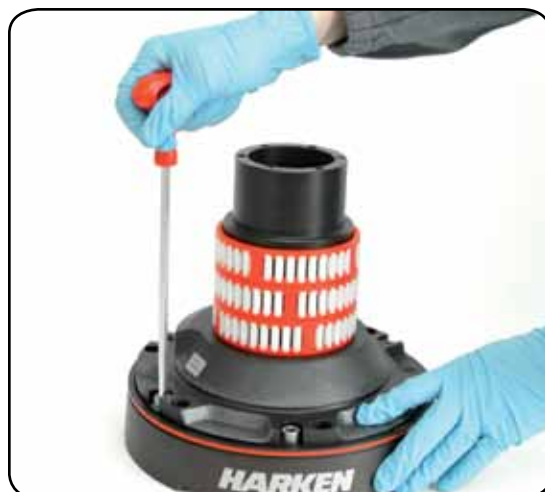
10. Unscrew the 6 hex screws n° 17 ( 20Nm/177 in-lb)
