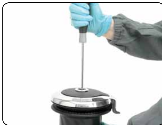
2. Unscrew the central screw ( \approx 2\text{Nm}/18\text{ in-lb} )
