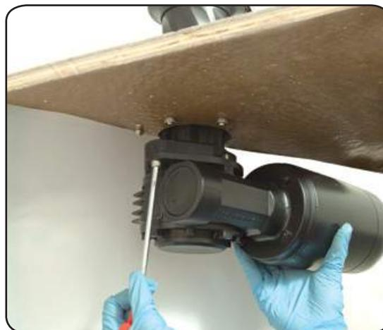
4. Tighten the two screws (8 Nm/ 71 in-lb).
