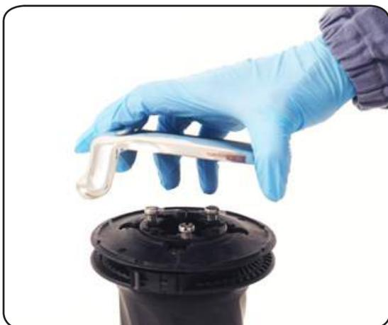
5. Remove the self-tailing arm n°28 by rotating and lifting it.
