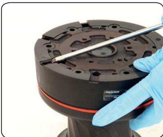
1. Remove the skirt n°2 with the help of the screwdriver placed as shown by the symbol
