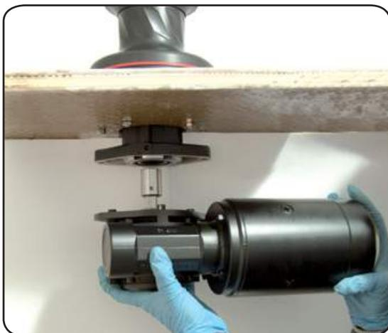
3. Position the reduction gear and motor
