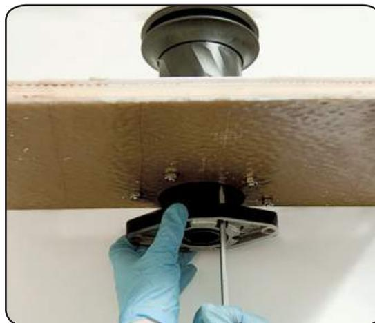
2. Tighten six M6 precote coated screws
