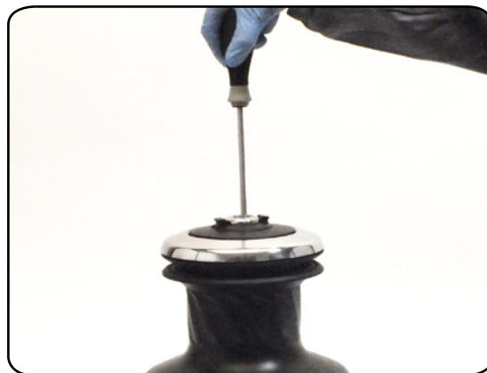
2. Unscrew the central screw ( \approx 2\text{Nm}/18\text{ in-lb} )
