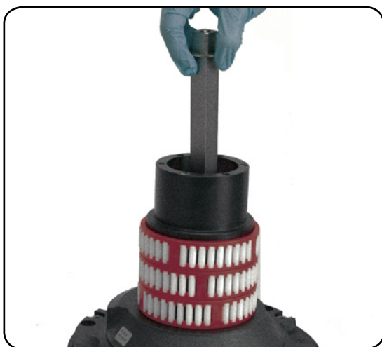
9. Slide out the central shaft n°19
