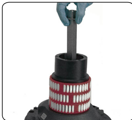
9. Slide out the central shaft n°19
