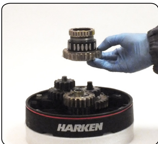
12. Remove the gear n°34, pawls carrier n°33, the bearings n°35 and 37 and the spring n°36
