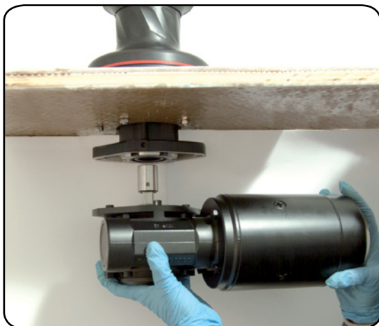
3. Position the reduction gear and motor
