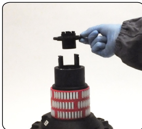
7. Remove the stripper arm housing n°21
