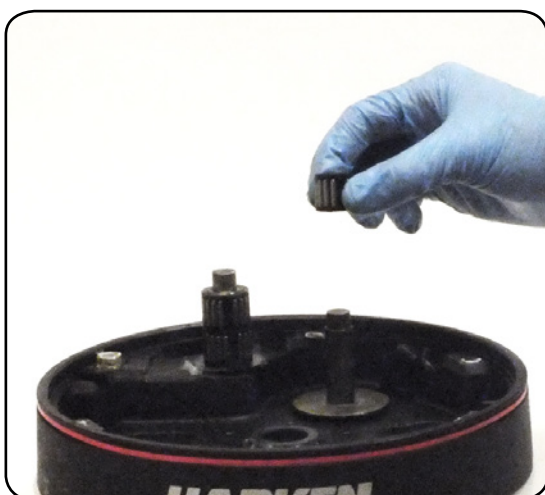
18. Remove the roller bearing n°12
