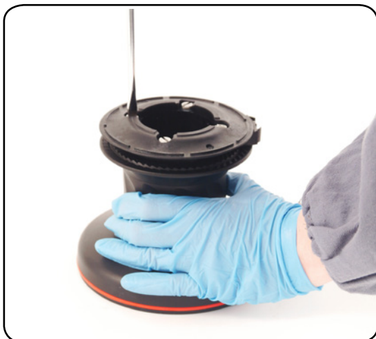
I. Unscrew the 4 screws n°26 (4Nm/35 in-lb)
