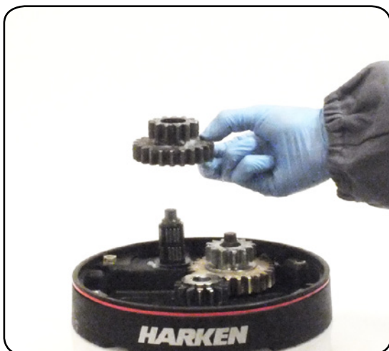
14. Remove the idler and pinion n°14
