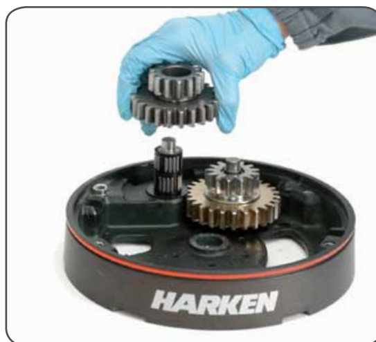
14. Remove the idler and pinion n°14
