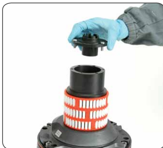
8. Remove the stripper arm housing n°21
