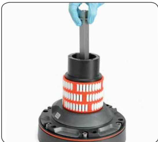
9. Slide out the central shaft n°19
