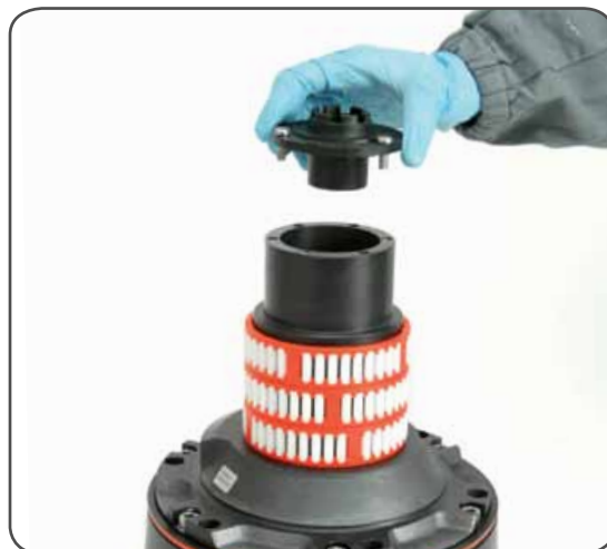
8. Remove the stripper arm housing n°21
