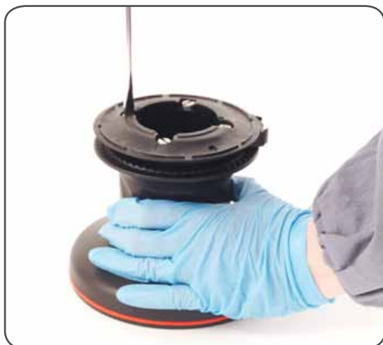
I. Unscrew the 4 screws n°26 ( \text{4Nm/35 in-lb} )
