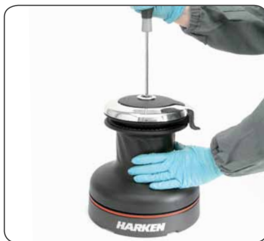
2. Unscrew the central screw ( \approx 2\text{Nm}/18\text{ in-lb} )
