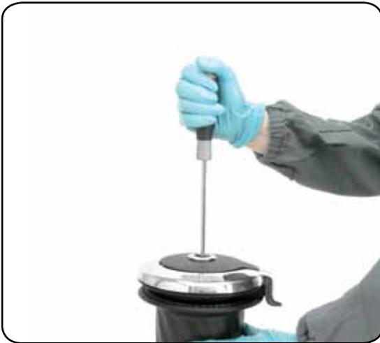
1. Unscrew the central screw ( $\approx 2\text{Nm}/18\text{ in-lb}$ )
