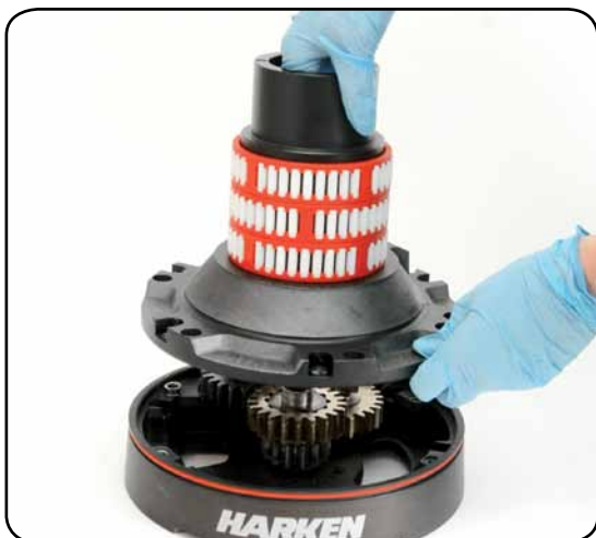
11. Remove the drum support n° 16
