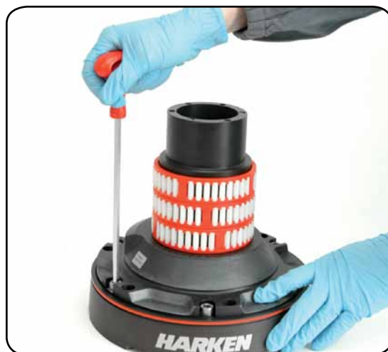
10. Unscrew the 6 hex screws n° 17 ( 20Nm/177 in-lb)
