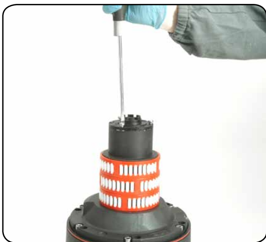
7. Completely unscrew the three screws n° 28
