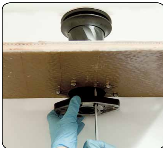
2. Tighten the six screws (8 Nm/ 71 in-lb)
