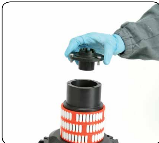
8. Remove the stripper arm housing n° 21
