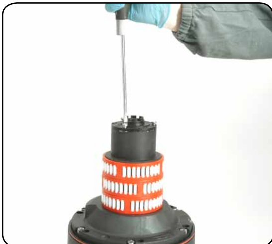
7. Completely unscrew the three screws n° 28
