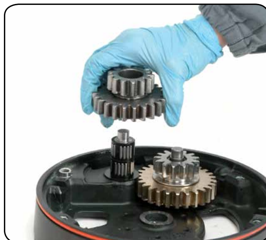
14. Remove the idler and pinion n°14
