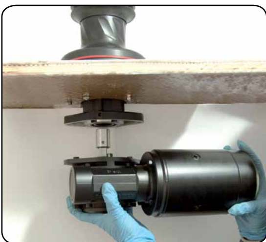
3. Position the reduction gear and motor
