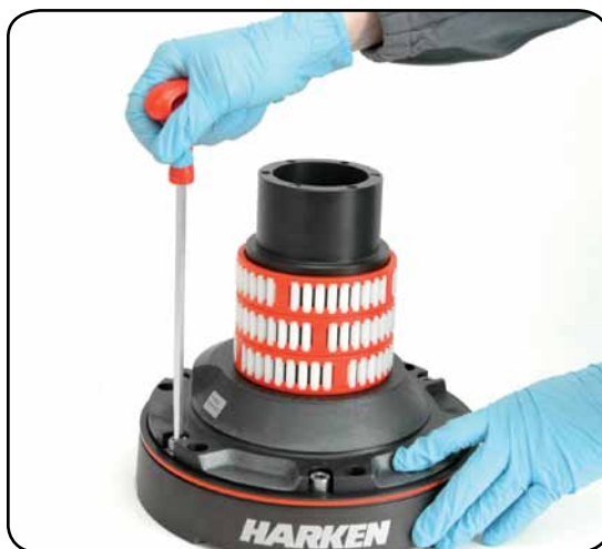
10. Unscrew the 6 hex screws n° 17 ( 20Nm/177 in-lb)
