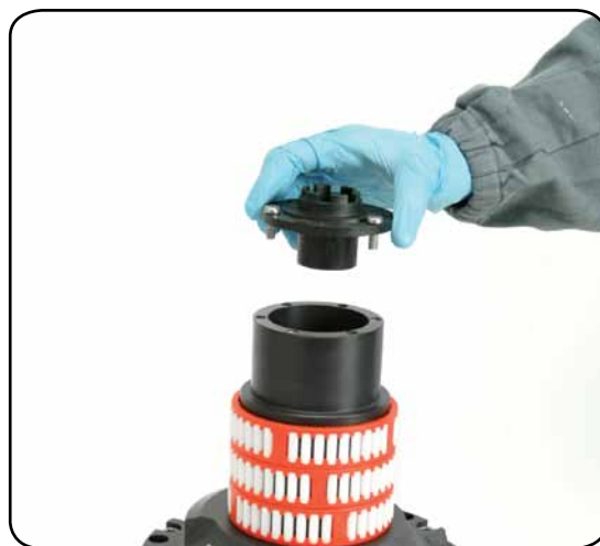
8. Remove the stripper arm housing n° 21
