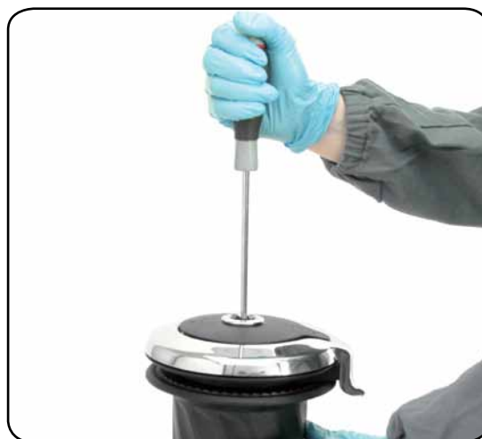
2. Unscrew the central screw ( \approx 2\text{Nm}/18\text{ in-lb} )
