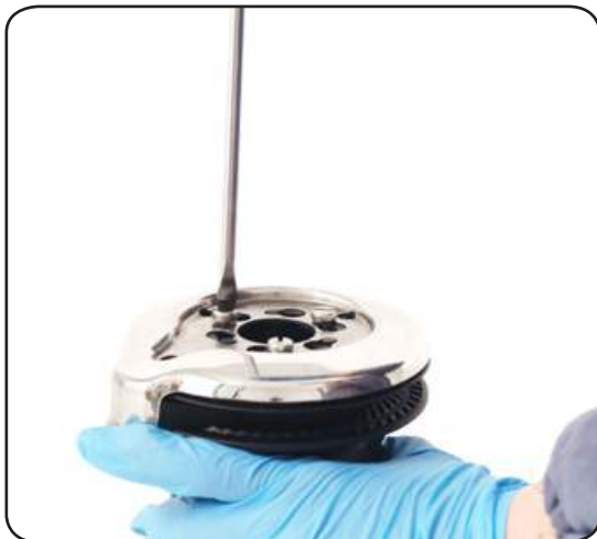
3. Unscrew the three screws n°27 ( \approx 4\text{Nm}/35\text{ in-lb} )
