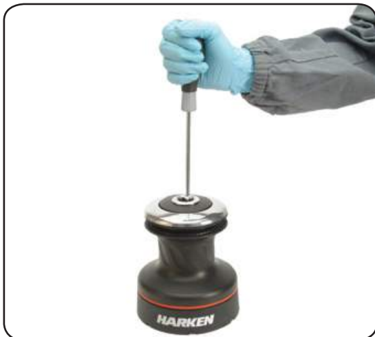
1. Unscrew the central screw ( \approx 2\text{Nm}/18\text{ in-lb} )
