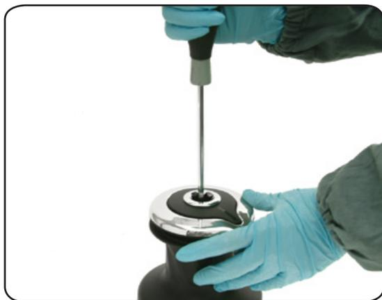
1. Unscrew the central screw ( $\approx 2\text{Nm}/18\text{ in-lb}$ )
