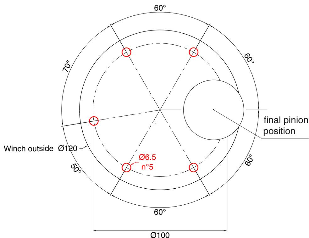
**B.** Remove the winch and drill the five 6.2 mm diameter holes.
