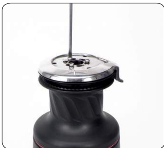
3. Unscrew the three screws n°25 (4Nm/35 in-lb) and remove the self-tailing arm n°8 by rotating and lifting it.
