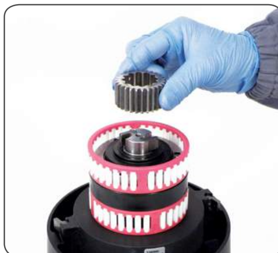
8. Lift off the gear n°9
