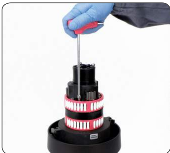
5. Unscrew the 6 hex screws n°18 (20Nm/177 in-lb)
