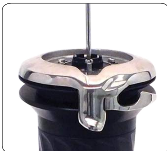
4. Unscrew the three screws n°41 (⌚ 4Nm/35 in-lb)
