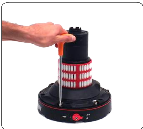
7. Unscrew the 6 hex screws n°14 ( \hookrightarrow 20Nm/177 in-lb)
