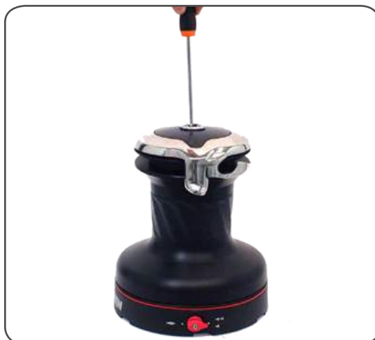
2. Unscrew the central screw (⌚ 2Nm/18 in-lb)
