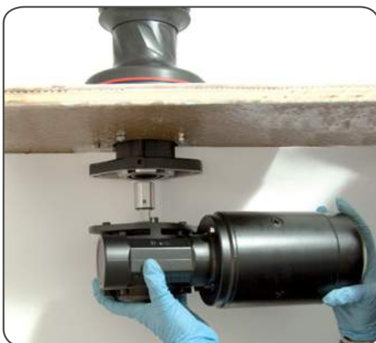
3. Position the reduction gear and motor
