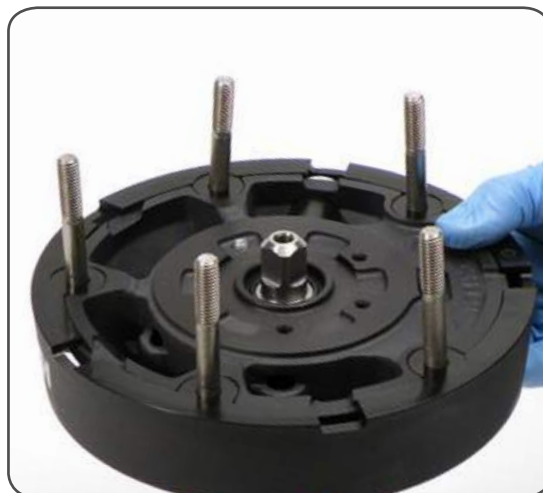
4. Reposition the skirt n°2 in its housing
