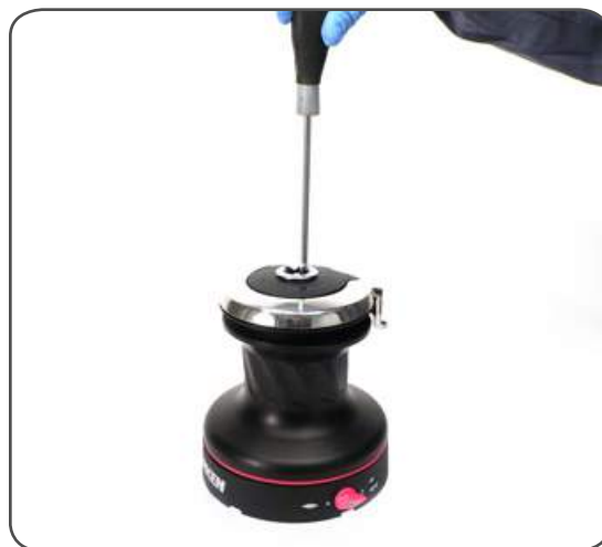
2. Unscrew the central screw ( \approx 2\text{Nm}/18\text{ in-lb} )
