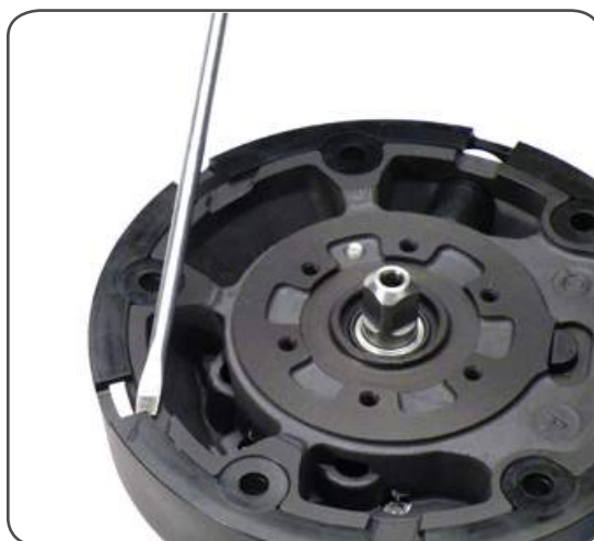
2. Remove the skirt n°2 with the help of the screwdriver placed as shown by the symbol
