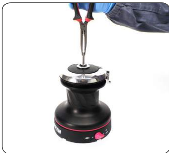
1. Pull out the disconnect rod n°28
