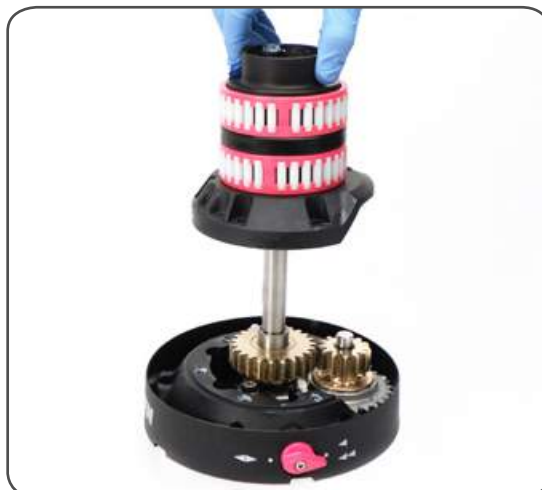
8. Remove the assy housing n°11
