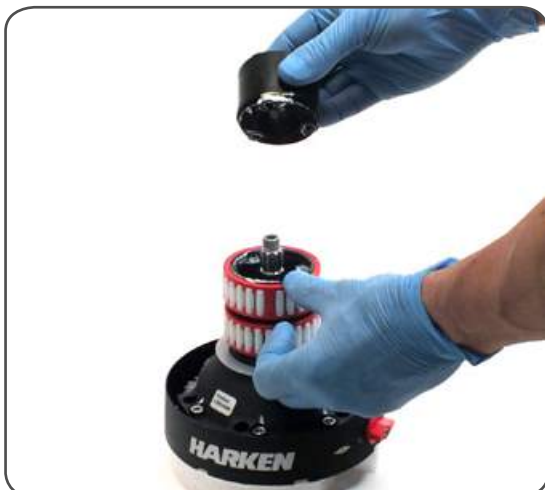
7. Remove the stripper arm support n°16
