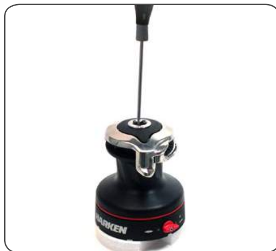
2. Unscrew the central screw ( \approx 2\text{Nm}/18\text{ in-lb} )
