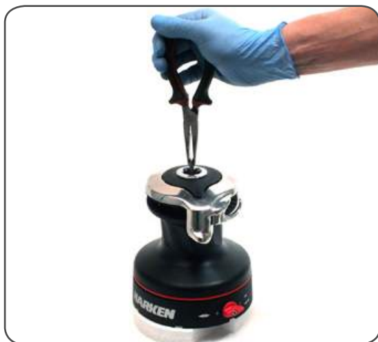
1. Pull out the disconnect rod n°31
