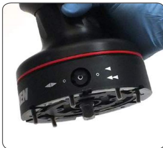
4. Reposition the skirt n°2 in its housing
