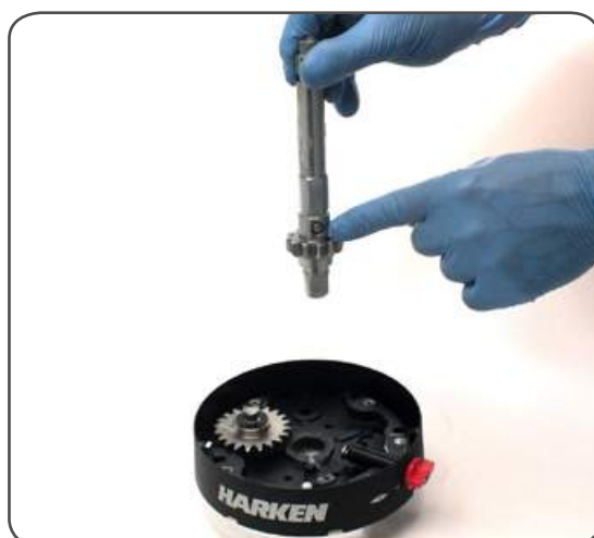
18. Slide out main shaft n°30 and pay attention to the two balls n°35
