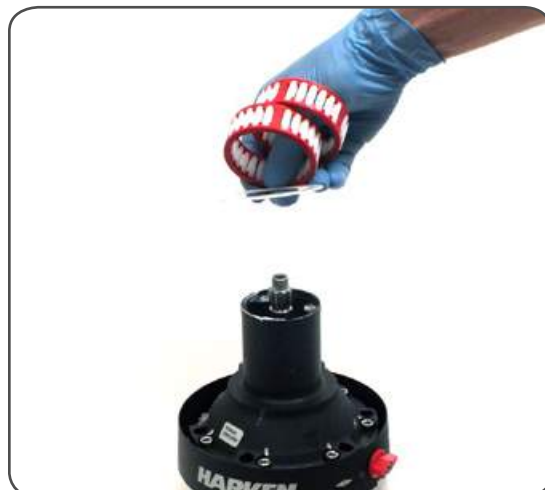
8. Slide out the bearings n°14 and the spacer n°13
