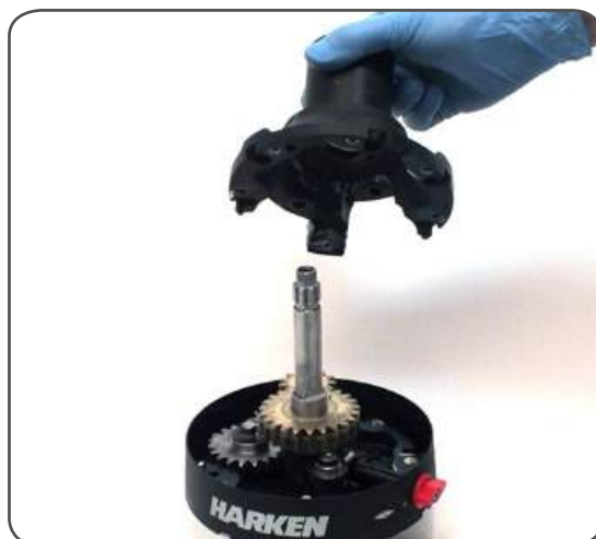
10. Remove drum support n°11
