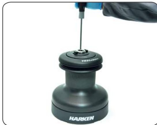
2. Unscrew the central screw ( \approx 2\text{Nm}/18\text{ in-lb} )
