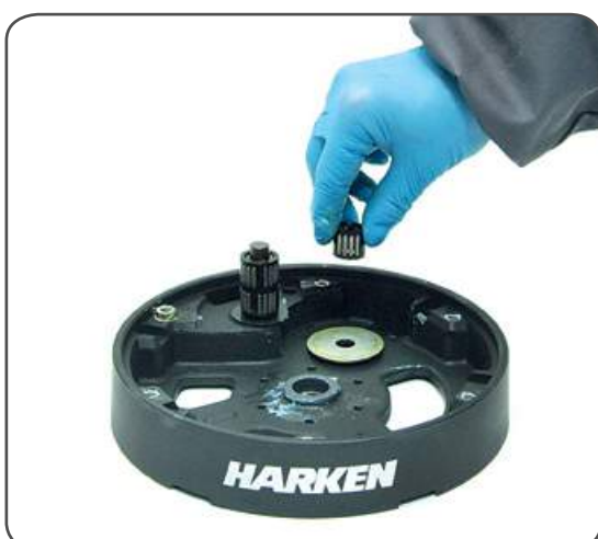
18. Remove the roller bearing n°12
