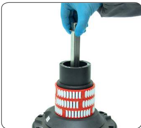
9. Slide out the central shaft n°19
