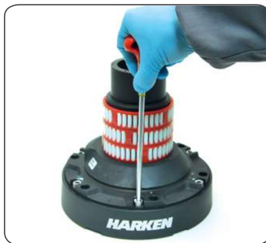
10. Unscrew the 6 hex screws n°17 (20Nm/177 in-lb)
