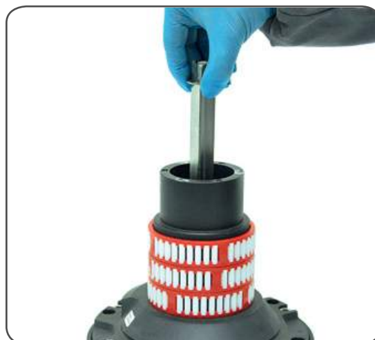
9. Slide out the central shaft n°19
