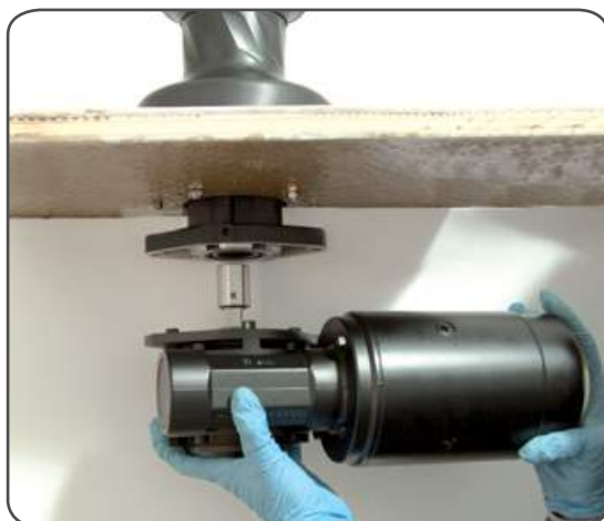
3. Position the reduction gear and motor
