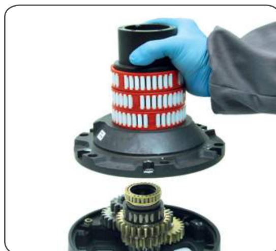
11. Slide out the drum support n°16
