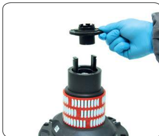
7. Remove the stripper arm housing n°21
