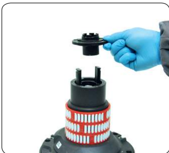
7. Remove the stripper arm housing n°21
