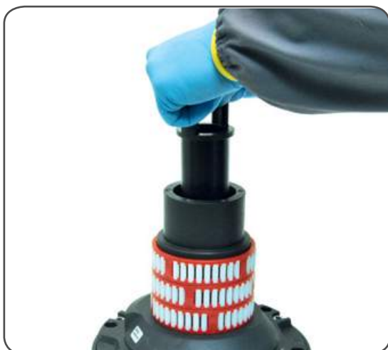
8. Slide out the assy clutch n°37
