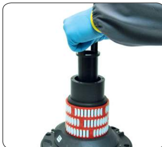
8. Slide out the assy clutch n°37
