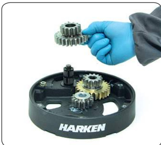
14. Remove the idler and pinion n°14
