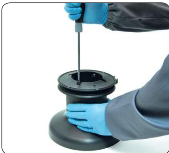
I. Unscrew the 4 screws n°25 (4Nm/35 in-lb)
