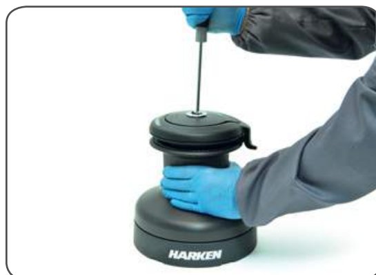
2. Unscrew the central screw ( \approx 2\text{Nm}/18\text{ in-lb} )
