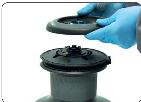
5. Remove the stripper arm n°26 by rotating and lifting it.
