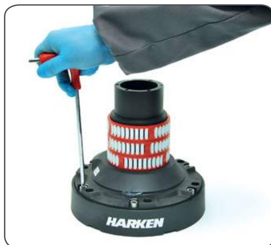
10. Unscrew the 6 hex screws n° 17 (🔧 20Nm/177 in-lb)
