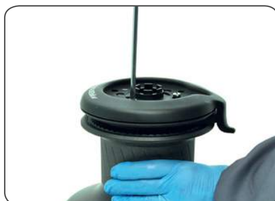
4. Unscrew the three screws n°27 ( \approx 4\text{Nm}/35\text{ in-lb} )
