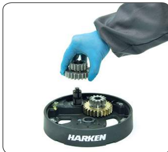
14. Remove the idler and pinion n°14.
