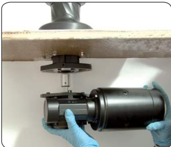
3. Position the reduction gear and motor
