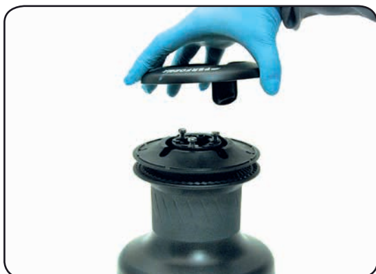
5. Remove the stripper arm n°24 by rotating and lifting it.
