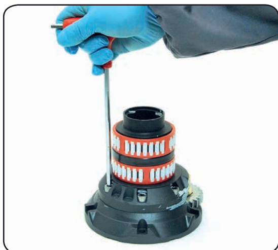
9. Unscrew the 5 hex screws n°16 ( \approx 20\text{Nm}/177\text{ in-lb} )
