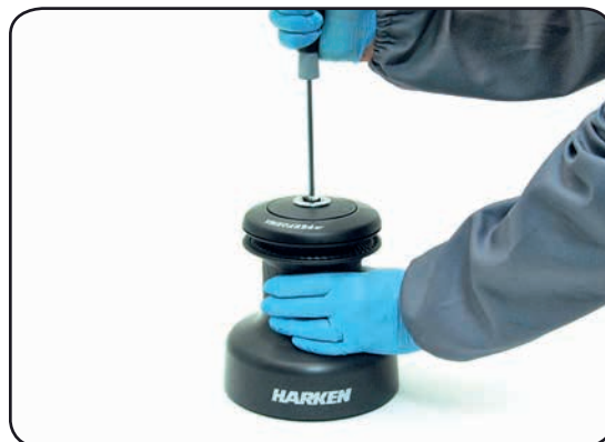
2. Unscrew the central screw ( \approx 2\text{Nm}/18\text{ in-lb} )
