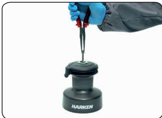
1. Pull out the disconnect rod n°28
