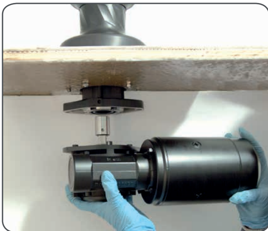
3. Position the reduction gear and motor
