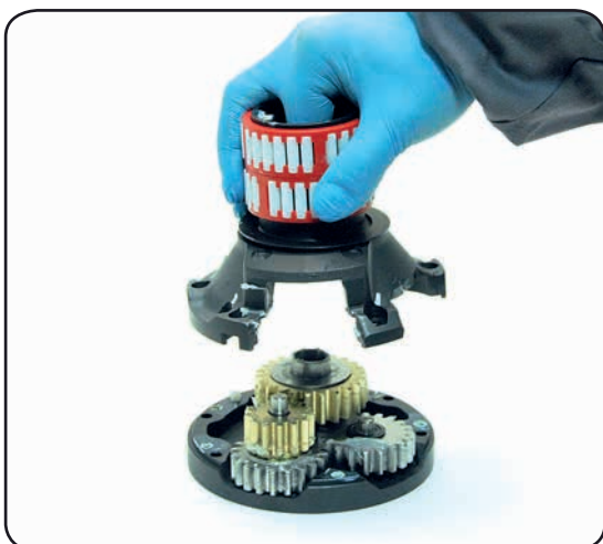
11. Remove the drum support n°14 Important: washer n°11 may remain inside the drum support!
