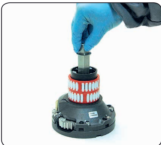
9. Slide out the central shaft n°18
