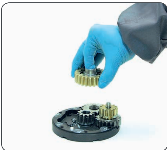
13. Remove the gearing n°6 and remove the pawls n°4. To facilitate the operation press the spring against the pawl with a blade.
