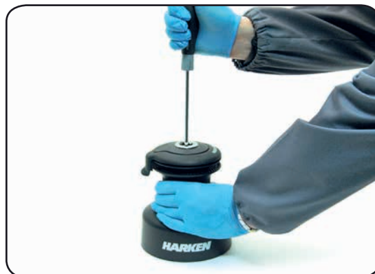
2. Unscrew the central screw ( \approx 2\text{Nm}/18\text{ in-lb} )
