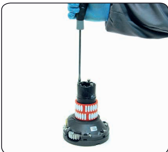
7. Completely unscrew the three screws n°25
