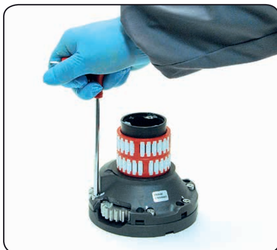
10. Unscrew the 6 hex screws n°15 (8Nm/71 in-lb)
