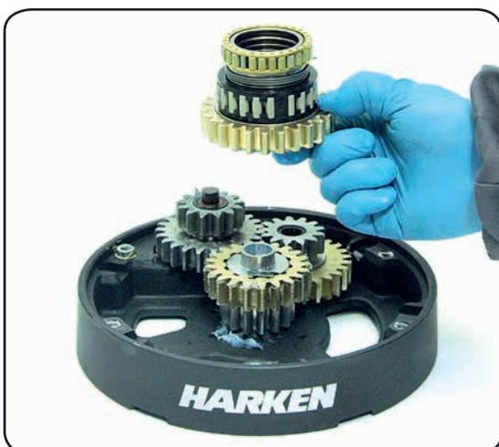
11. Remove gear n°32, pawls carrier n°31, the bearings n°33 and 35 and the clutch spring n°34.
