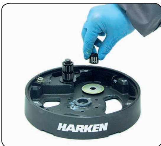
17. Remove the roller bearing n°12
