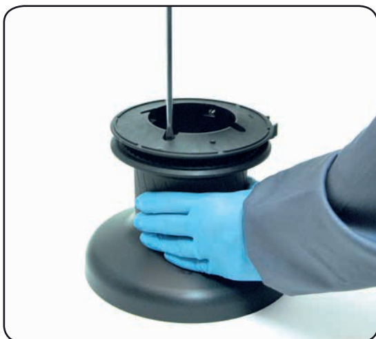
I. Unscrew the 4 screws n°24 (4Nm/35 in-lb)
