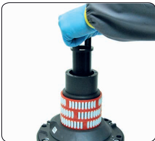
7. Slide out the assy clutch n°35
