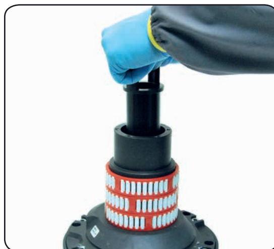
7. Slide out the assy clutch n°35
