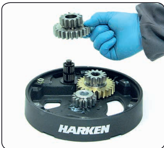
13. Remove the idler and pinion n°14
