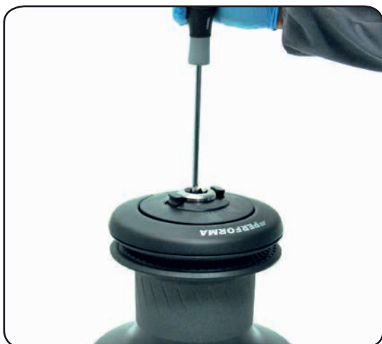
1. Unscrew the central screw (⚙️ 2Nm/18 in-lb)
