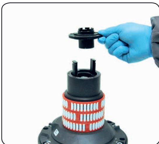
6. Remove the stripper arm housing n°21
