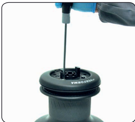
3. Unscrew the three screws n°26 (⚙️ 4Nm/35 in-lb)
