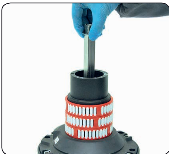
8. Slide out the central shaft n°19
