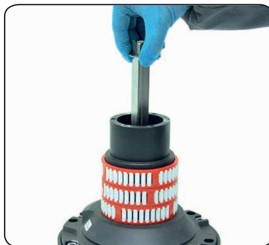
8. Slide out the central shaft n°19
