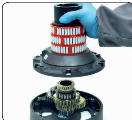
10. Slide out the drum housing n°16. Attention! The gear assembly n°36 remains inside the drum housing
