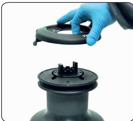
4. Remove the stripper arm n°25 by rotating and lifting it.
