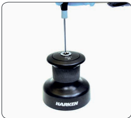
1. Unscrew the central screw (⚙️ 2Nm/18 in-lb)
