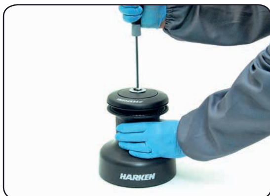
1. Unscrew the central screw ( \approx 2\text{Nm}/18\text{ in-lb} )
