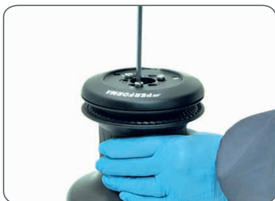
3. Unscrew the three screws n°25 ( \approx 4\text{Nm}/35\text{ in-lb} )
