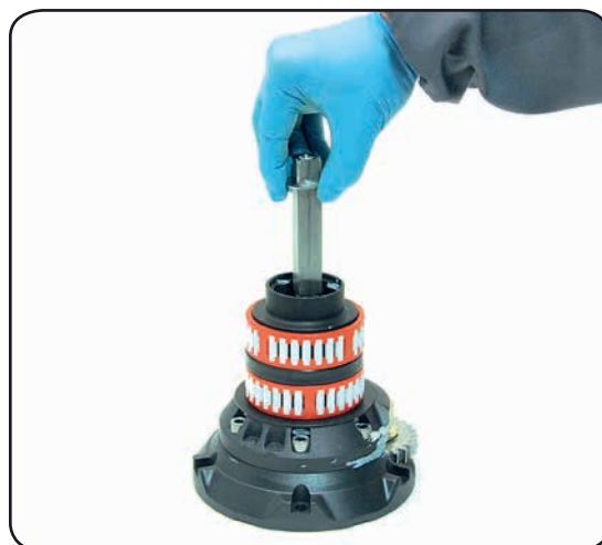
7. Slide out the central shaft n°19
