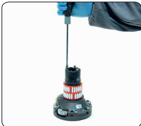
6. Completely unscrew the three screws n° 24
