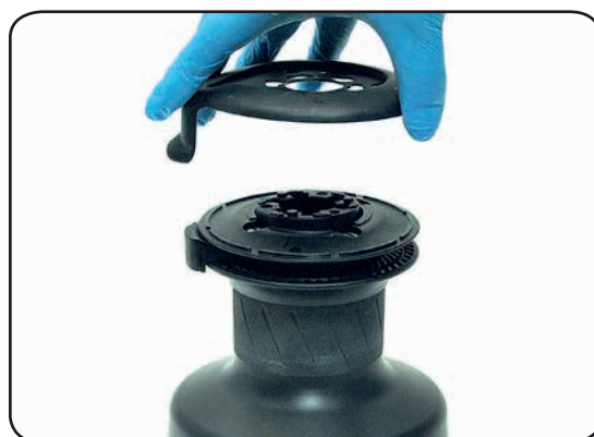
4. Remove the stripper arm n°28 by rotating and lifting it.
