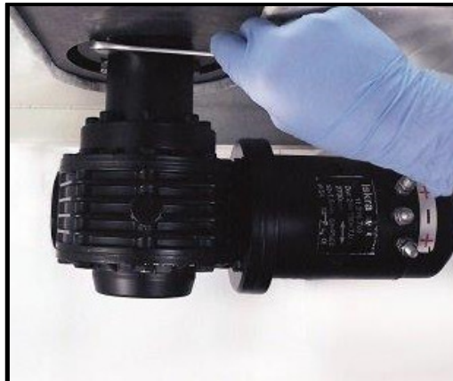
L. Tighten the four M10 screws (20Nm/177 in-lb)
