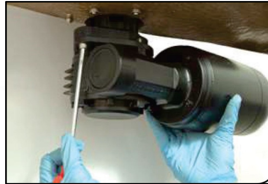
H. Tighten six M6 precote screws (8Nm/71 in-lb)
