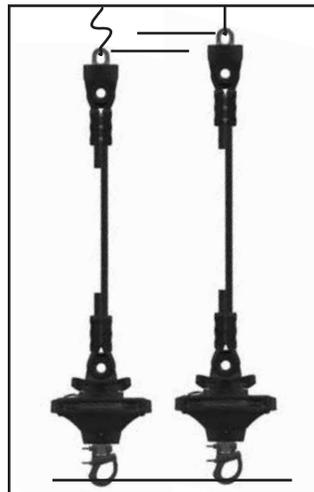
Note: When using an A2 sail, it is important to maximize the cable length so the sail can be at full hoist. The best way to achieve the maximum is to add to the cable length, then adjust the cable length after sailing. When sailing, tension the halyard only enough to pull slack out of the Reflex torsion cable.
