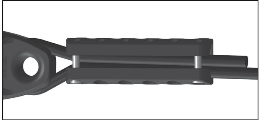
6. Continue to tighten the four (4) long corner fasteners until the gap between the clamp halves is around 5 mm (3/16"). Now tighten the eight (8) center fasteners until snug.
