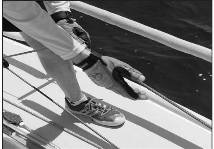
Continue furling by easing the sheet part way and furling so flogging is minimized and there is some drag on the sheets. Furl until the clew pennant or sheets are securely wrapped around the furled sail.
