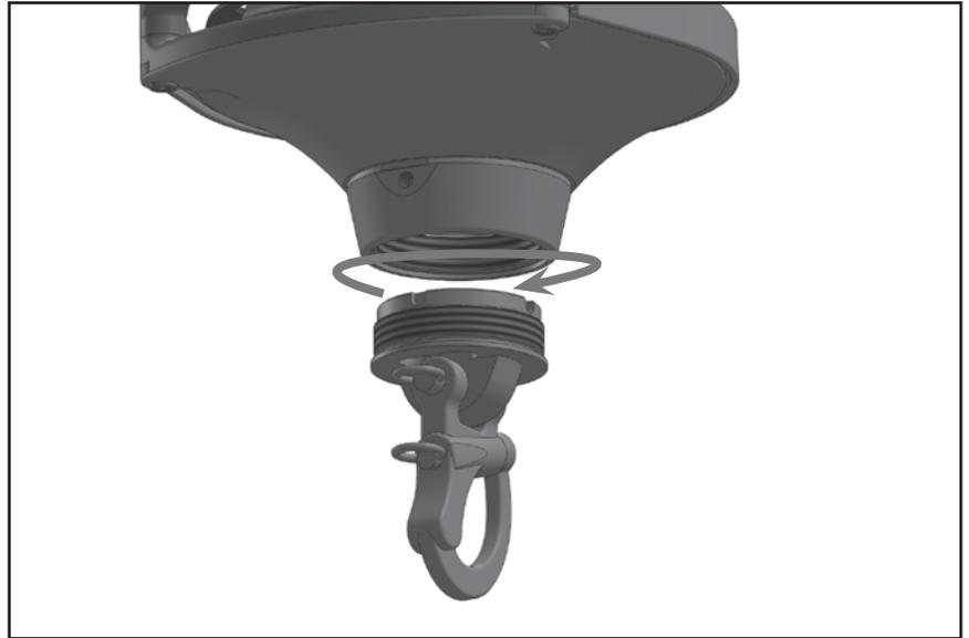
Back the adapter out no more than one (1) rotation until the set screw holes line up with the recesses at the top of the threaded adapter. Sight into one of the set screw holes to confirm alignment.
