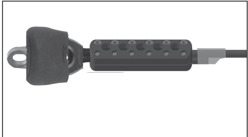
10. If assembling away from the boat, lay cable out straight. Install tack terminal and snap shackle adapter on drive unit. **Note:** See following pages for preferred method of determining length at boat.
