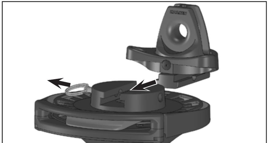
**2. Finding cut length:** Attach the lower unit assembly to the tack line or fixed bail and pull the tack line all the way down. Slip the bottom of the cable through the thimble in the tack terminal. Pull the cable as tight as you can **by hand**, and wrap a piece of electrical tape **where the cable enters the thimble**. This is point A. Point A will likely be the cut point. Cable stretch will account for the distance around the thimble and the clamp height.
