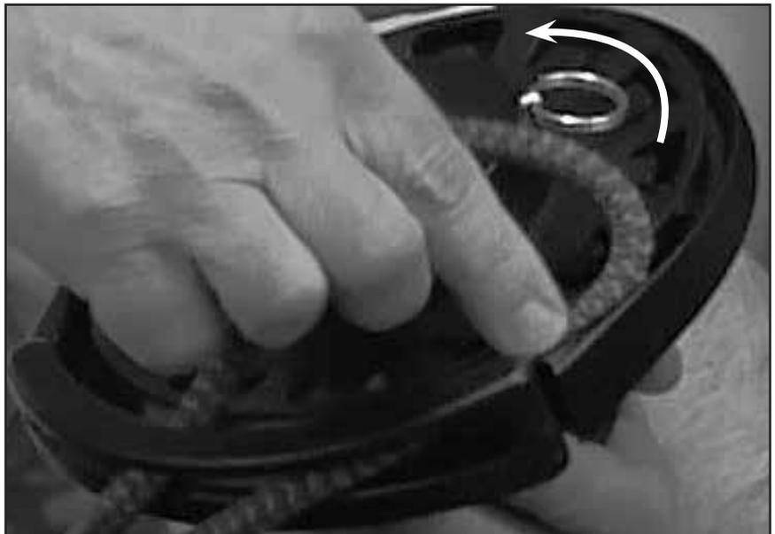
Rotate the drive sheave as you press the line into position around the drive sheave. Load the final part by pulling the line from outside the drive unit.
