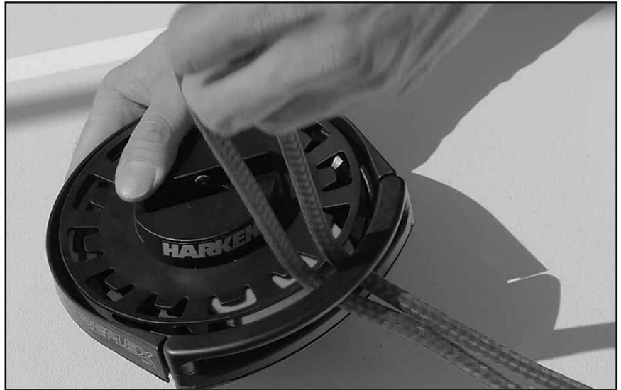
Work the line into the space between the drive sheave and the flexible cowling.
