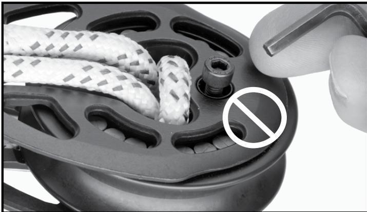
3. Inspect loops and lashings. Replace if there are signs of wear, or if the colored tracer fades from UV damage. Pull loop out of mouth and inspect loop/lashing carefully for any signs of wear, UV damage, fatigue, or strand separation. Replace loop if it shows signs of UV damage or wear.
