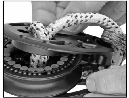
**Tip:** With shorter loops, place loop at the side of the head to allow more room to insert the deadend post.
