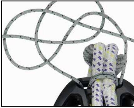
10. Further secure knot by carefully melting line ends with a hot knife.
