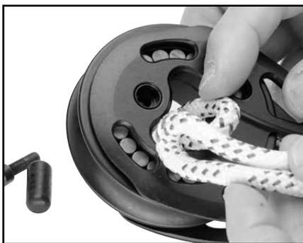
4. Pass loop ends through mouth so loops extend beyond block's sideplates as shown.
