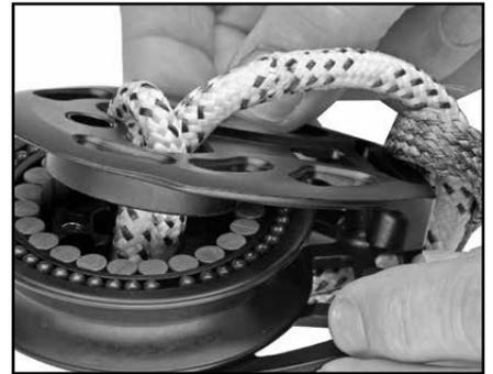
**Tip:** With shorter loops, place loop at the side of the head to allow more room to insert the deadend post.
