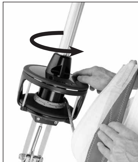
Sun cover on port side: wrap line by turning counterclockwise
