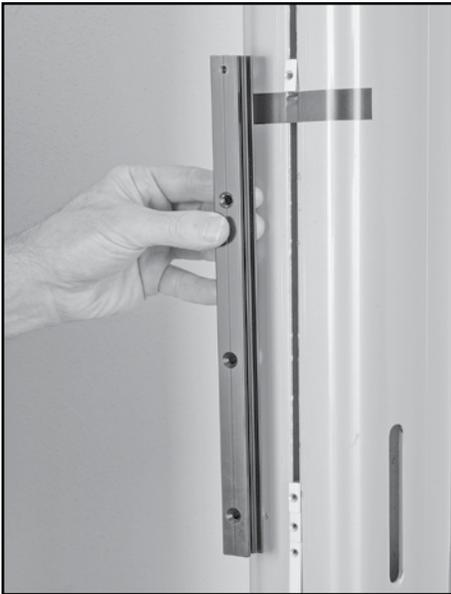
Slip top track slugs into mast groove. Use 32 mm (3/4") mounting slug for top stop.
