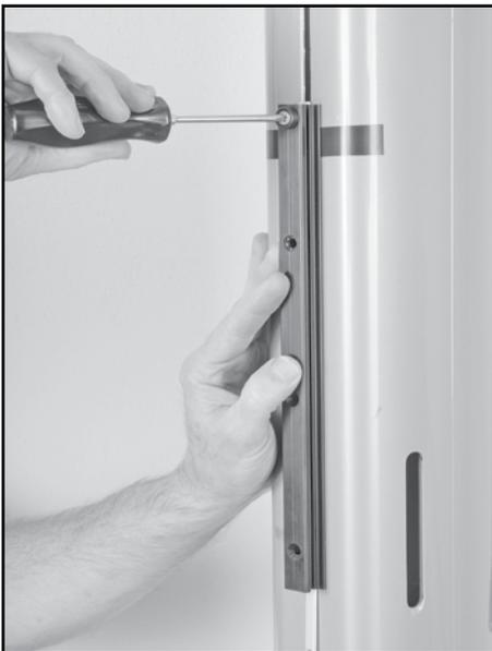
Thread 5 mm x 25 mm endstop screw through endstop, track, and into slug.
