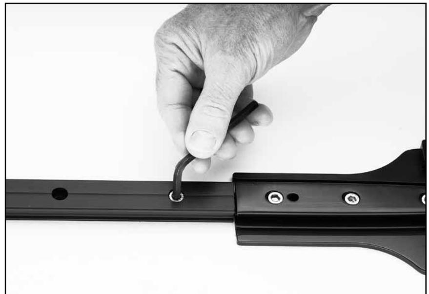
With track off mast, tap upper splice link into track using procedures outlined above.
