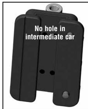
If cars are off track and sail attaching hardware removed, do not mix intermediate base cars with batten or headboard base cars. All cars have center hole in aluminum car. Low friction sliders have a hole in the plastic visible from below and from hole in aluminum car.
