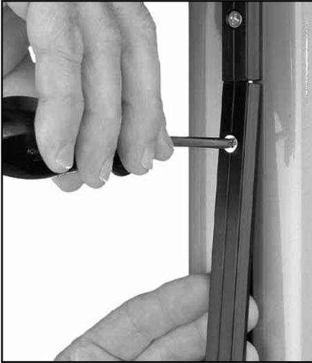
Hold full-length track piece up to mast. Loosely install top screw.
