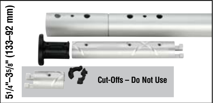
5 1/4"–3 5/8" (133–92 mm) Do not use plastic bushing above top connector. Cut connector right at cross formed by glue dispersion channels. Use single foil screw in top foil only.
