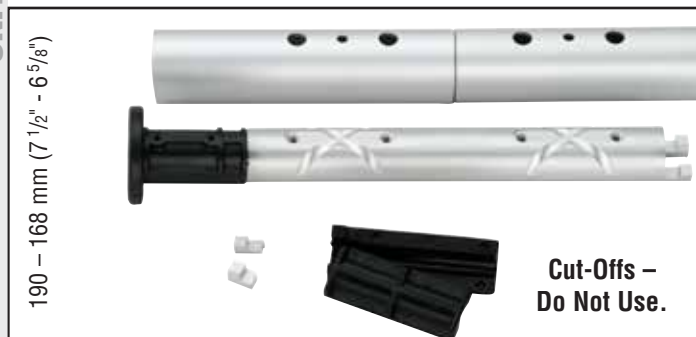
190 - 168 mm (7 1/2" - 6 5/8") Do not use plastic bushing above top connector. Shorten top of connector and if necessary shorten trim cap.
