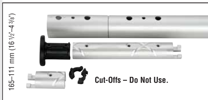
165 - 111 mm (6 1/2" - 4 3/8") Do not use plastic bushing above top connector. Cut connector right at cross formed by glue dispersion channels. Use single foil screw in top foil only.
