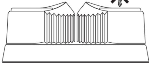
**Note: 412/420 double-wide cam cleat requires notches in 144/205 swivel arm for installation.**
