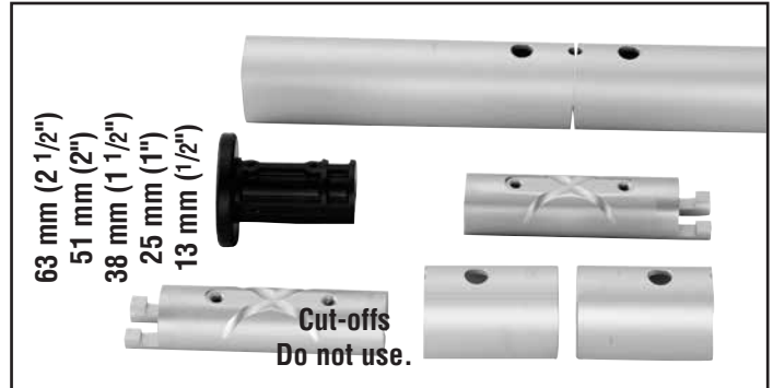
63 - 13 mm (2 1/2" - 1/2") . Shorten top foil and adjoining full-length foil so two (2) screws are used to assemble joint instead of four (4). Do not use plastic bushings above top connector.
