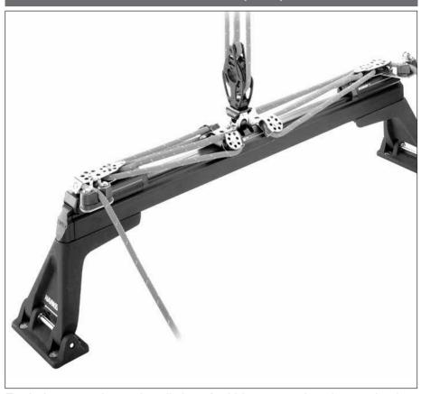
Track risers permit easy installation of mid-boom travelers that need to be raised to clear companionway hatches.
