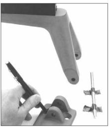
Mark outer two holes of each track riser base.
