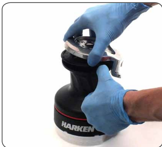
5. Remove the stripper arm n°21 by rotating and lifting it.
