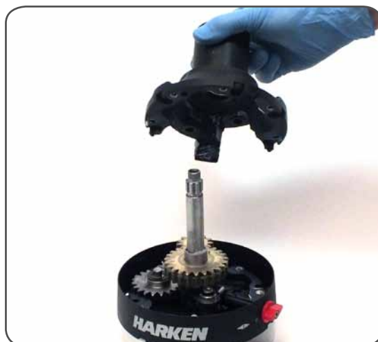
10. Remove drum support n°11
