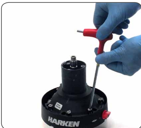
9. Unscrew the 6 hex screws n°12 ( \approx 20\text{Nm}/177\text{ in-lb} )
