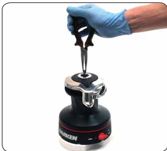
1. Pull out the disconnect rod n°31
