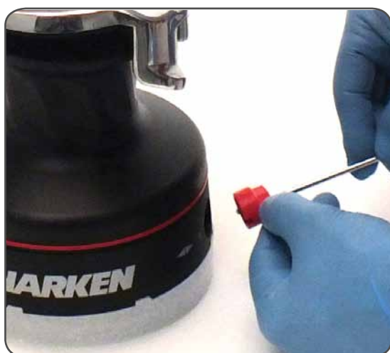
1. Unscrew the screw n°26 and slide off the knob n°24 (0,5 Nm/ 4,42 in-lb)
