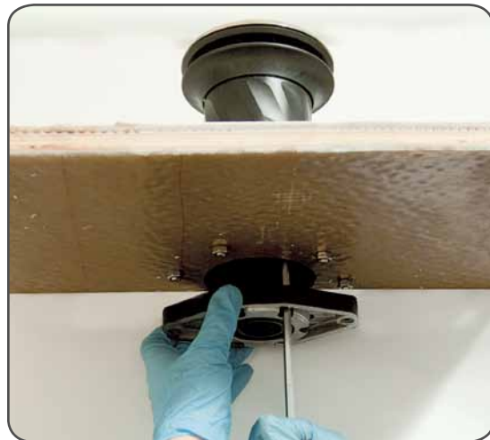
2. Tighten six M6 precote coated screws (8 Nm/ 71 in-lb)
