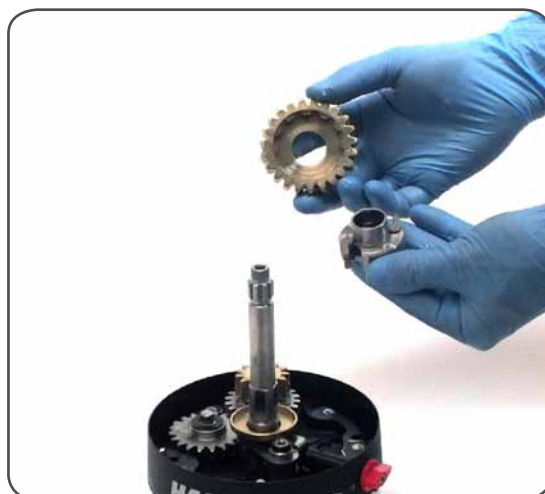
12. Remove pawls carrier n°33. Pay attention to the springs.
