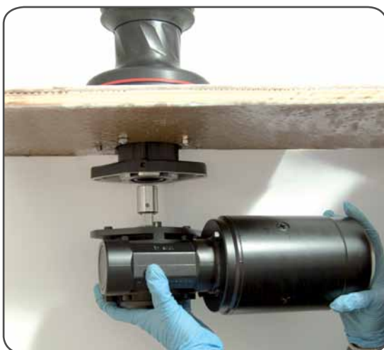
3. Position the reduction gear and motor
