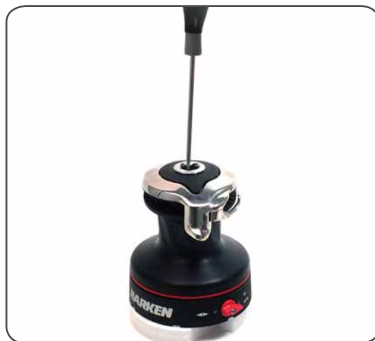
2. Unscrew the central screw ( \approx 2\text{Nm}/18\text{ in-lb} )
