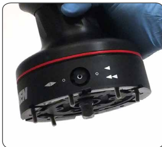
4. Reposition the skirt n°2 in its housing
