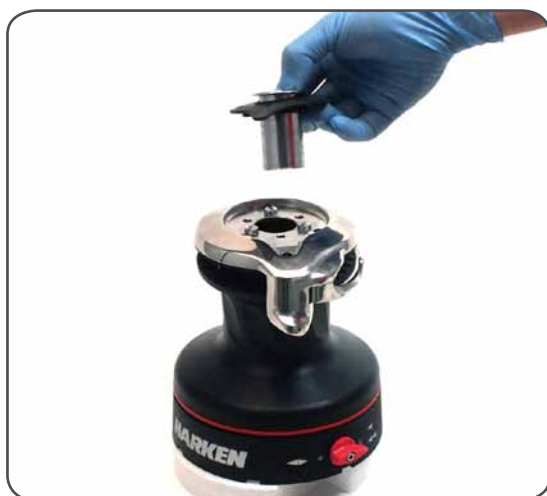
3. Slide off the assy socket n°25 and the cover n°20. Pay attention to the o-ring in the socket.
