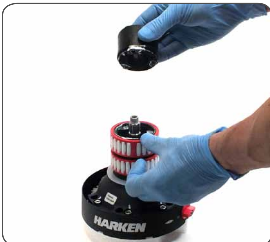
7. Remove the stripper arm support n°16
