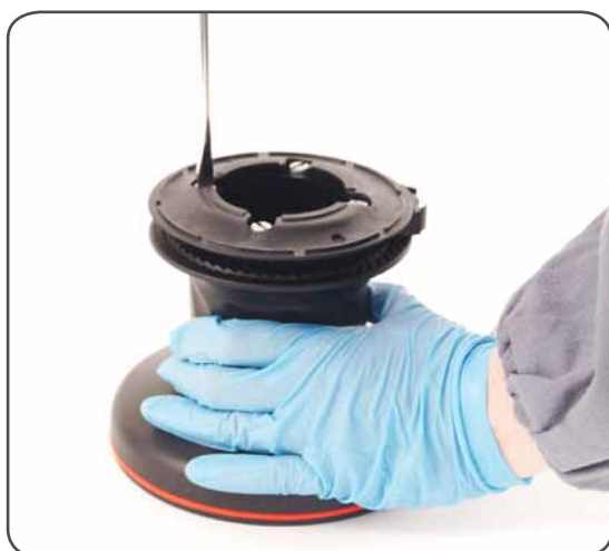
I. Unscrew the 4 screws n°18 (4Nm/35 in-lb)
