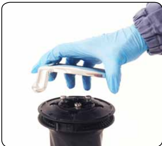
5. Remove the self-tailing arm n°26 by rotating and lifting it.
