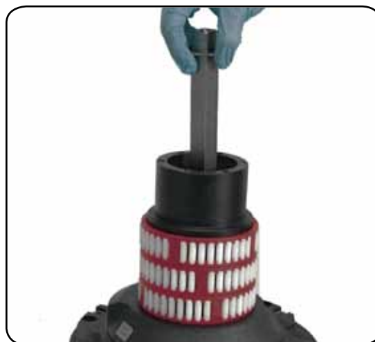
9. Slide out the central shaft n°19
