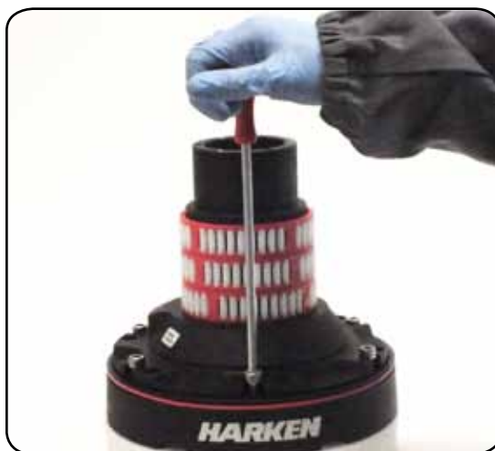
10. Unscrew the 6 hex screws n°17 ( \hookrightarrow 20Nm/177 in-lb)
