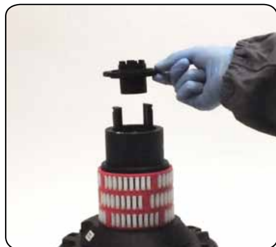
7. Remove the stripper arm housing n°21
