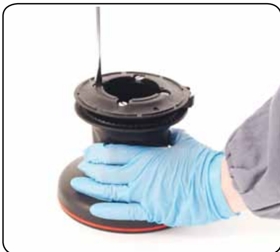
I. Unscrew the 4 screws n°26 (4Nm/35 in-lb)
