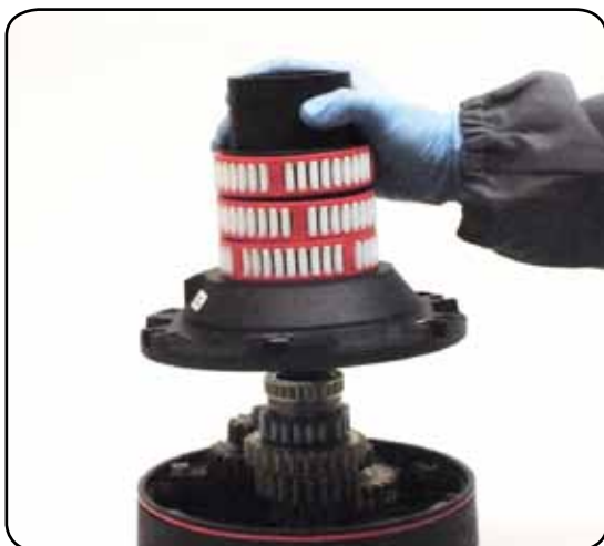
11. Remove the drum support n°16
