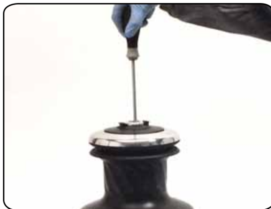
2. Unscrew the central screw ( \approx 2\text{Nm}/18\text{ in-lb} )
