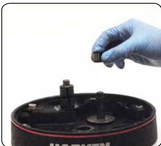
18. Remove the roller bearing n°12
