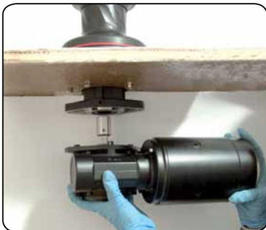
3. Position the reduction gear and motor
