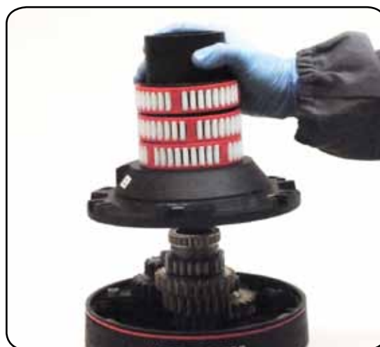
11. Slide out the drum support n°16
