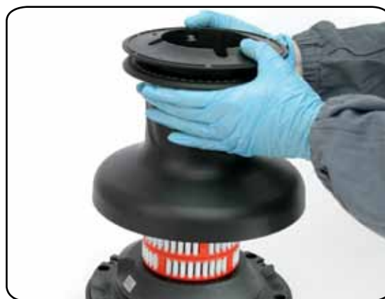
6. Lift off the drum n°24
