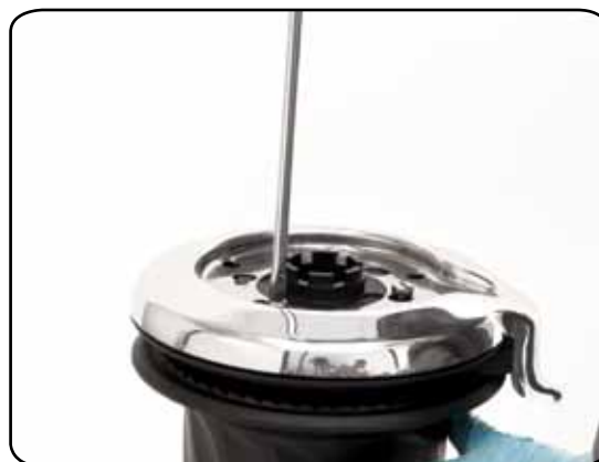
4. Unscrew the three screws n°28 ( \approx 4\text{Nm}/35\text{ in-lb} )
