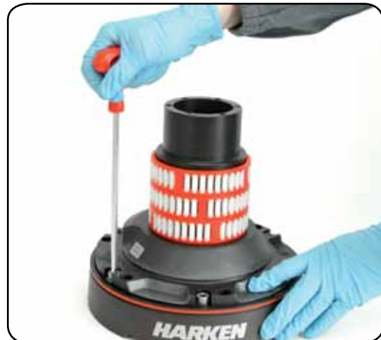
10. Unscrew the 6 hex screws n°17 ( 20Nm/177 in-lb)
