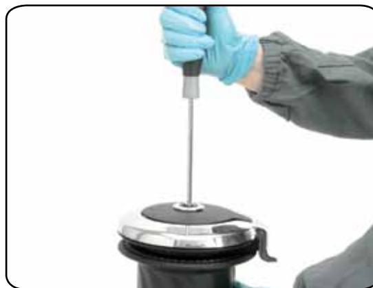
2. Unscrew the central screw ( \approx 2\text{Nm}/18\text{ in-lb} )
