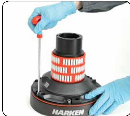
10. Unscrew the 6 hex screws n°17 ( 20Nm/177 in-lb)
