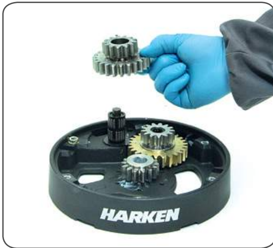
14. Remove the idler and pinion n°14
