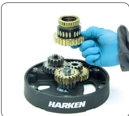
12. Remove the gear n°30, pawls carrier n°32, the bearings n°33 and 35 and the pin n°34 Important: washer n°7 may remain inside the drum support!
