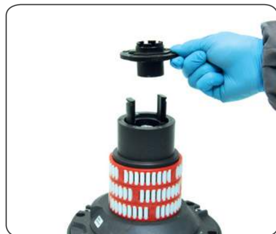
7. Remove the stripper arm housing n°21
