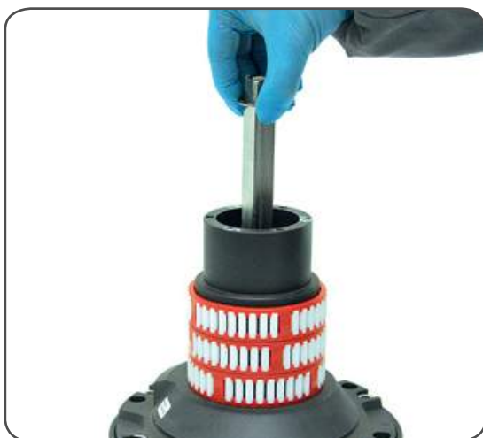
9. Slide out the central shaft n°19
