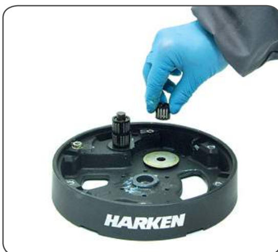
18. Remove the roller bearing n°12
