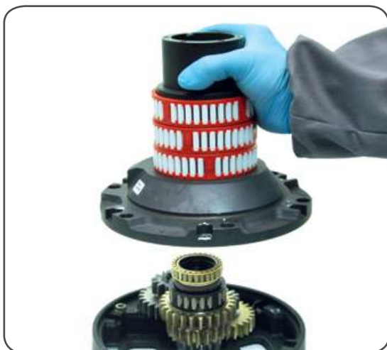
11. Remove the drum support n°16
