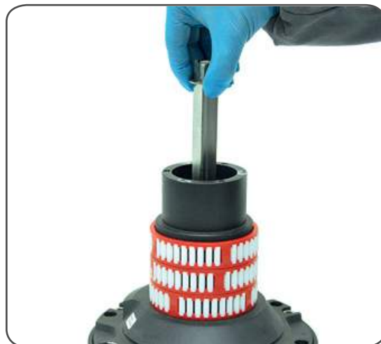
9. Slide out the central shaft n°19
