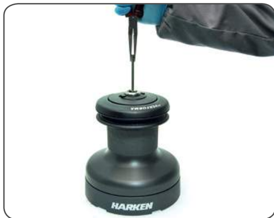
1. Pull out the disconnect rod n°37
