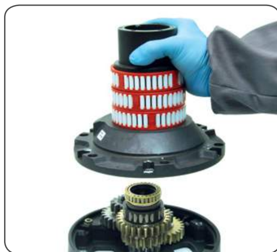
11. Slide out the drum support n°16
