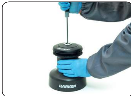
2. Unscrew the central screw ( \approx 2\text{Nm}/18\text{ in-lb} )
