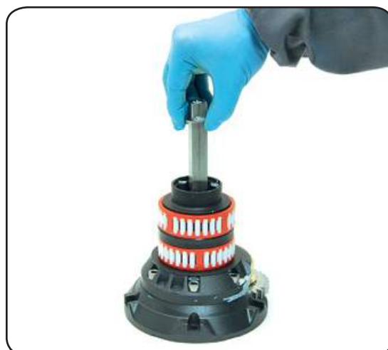
8. Slide out the central shaft n°20
