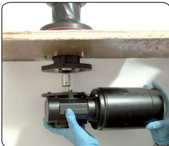
3. Position the reduction gear and motor
