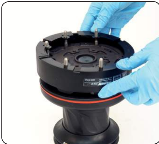
4. Reposition the skirt n°2 in its housing
