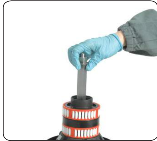
7. Slide out the central shaft n°21
