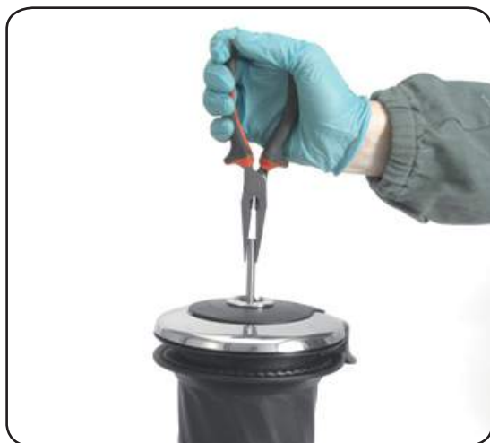
1. Pull out the disconnect rod n°32
