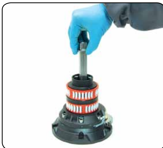
8. Slide out the central shaft n°19
