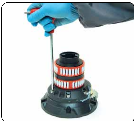
9. Unscrew the 5 hex screws n°16 (20Nm/177 in-lb)
