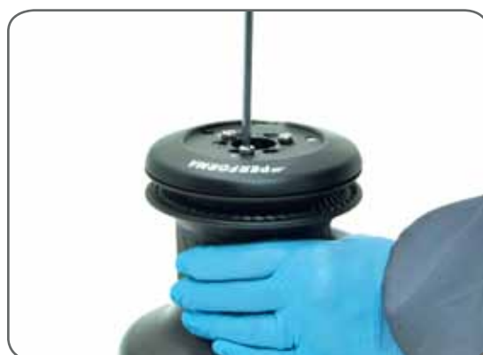
4. Unscrew the three screws n°25 ( \approx 4\text{Nm}/35\text{ in-lb} )
