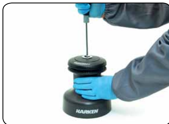
2. Unscrew the central screw ( \approx 2\text{Nm}/18\text{ in-lb} )
