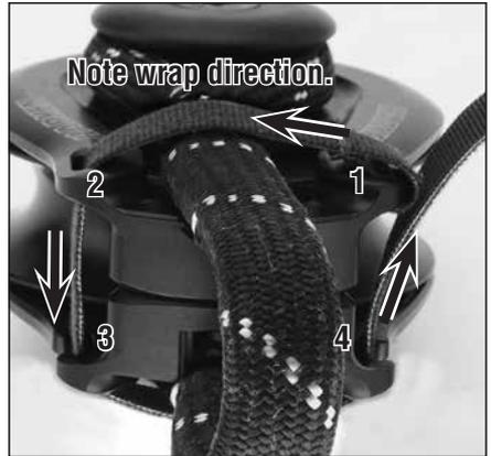
6. Pull the Velcro band tightly as you wrap. Note: there is no need to pass the Velcro band through the closed slot on the band's second pass. Make sure the band is securely seated in the open slots on the beta cheek. Press band in place to secure Velcro, and tuck the reflective band into open slots.
