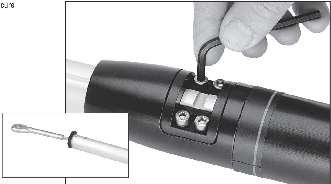
Slide halyard swivel above feeder. Place feeder in foil recess. Push screw down so tab catches under foil. Tighten screw.
