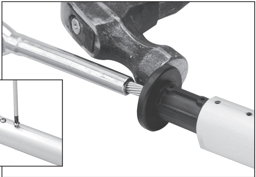
Place halves of plastic bushings on stay so hooked part of longer section faces out.
