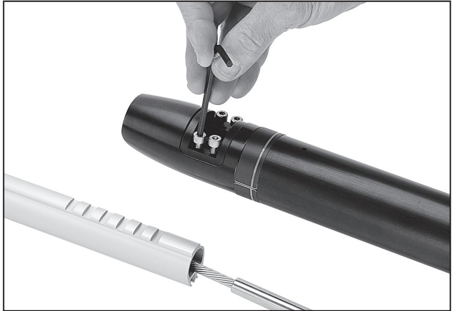
Slide drum assembly onto foils.
