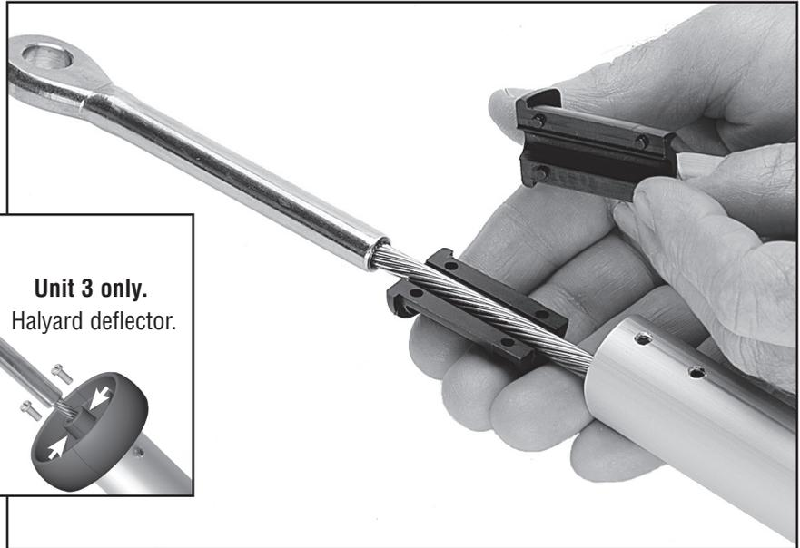
Push trim cap into foil to start; tap in using hammer.
