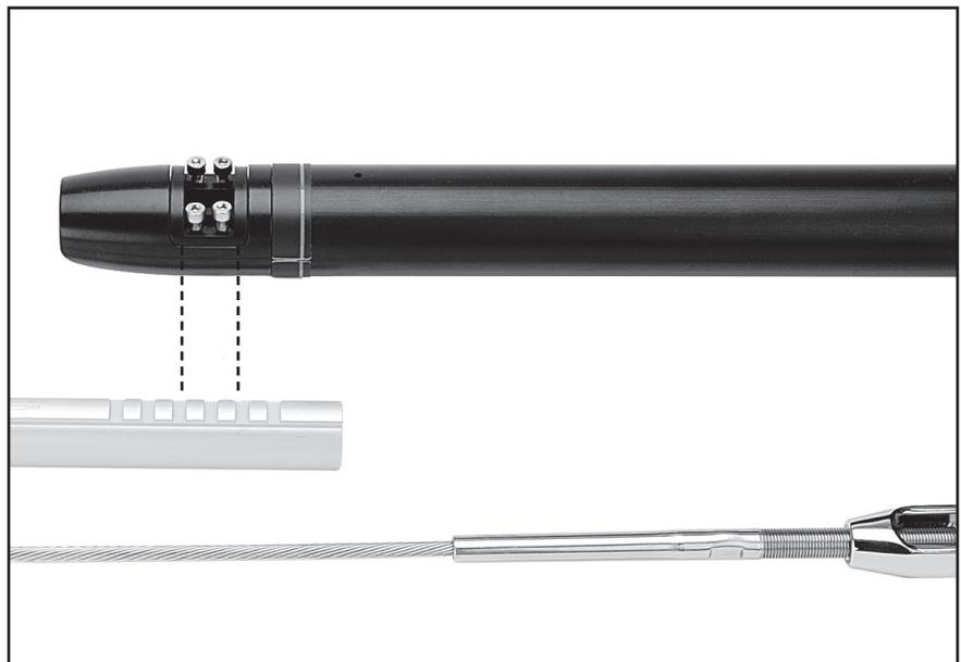
**Note:** Position top foil so that including top cap, the foil will ride 25 mm (1") below terminal. If wire fitting at top of stay is swage, foil must ride just below shoulder of swage. Mark cut line on foil. Wrap tape around foil as a guide so cut is straight.
