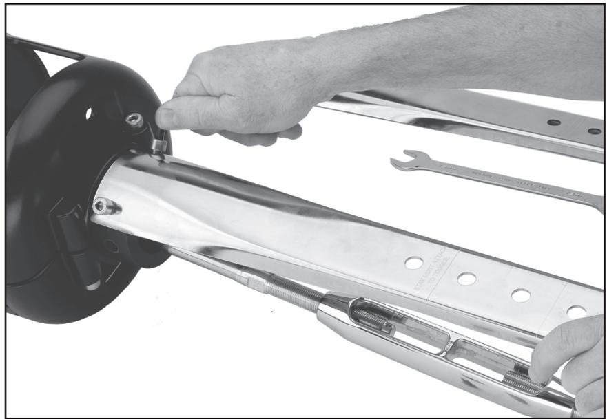
Fasten second long link plate to drum assembly and secure to toggle using locknuts.
