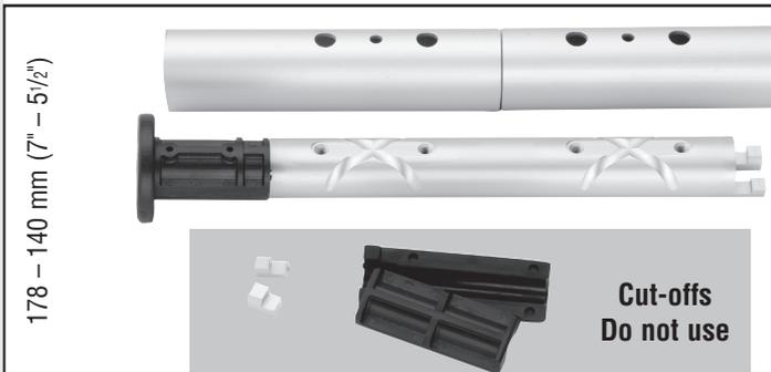
**178 – 140 mm (7" – 5 1/2")** Do not use plastic bushing above top connector. Shorten top of connector and, if necessary, shorten trim cap.
