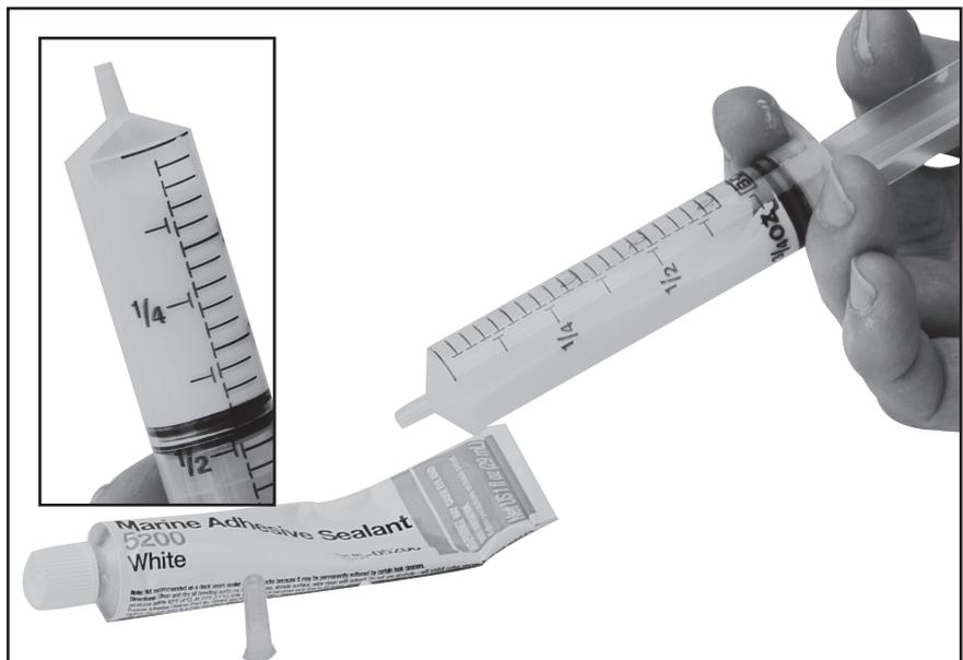
Inject only a small amount of adhesive into middle hole.
