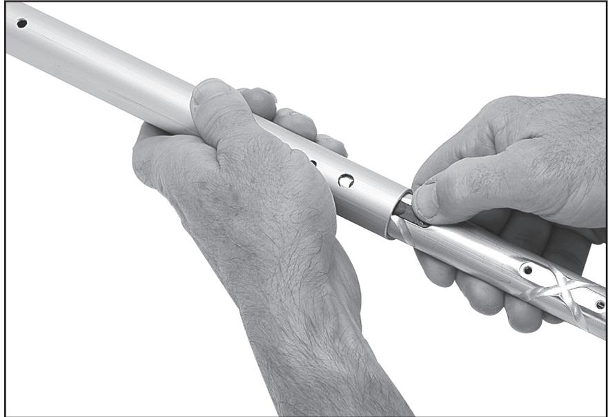
**Loading Injector with Adhesive**
