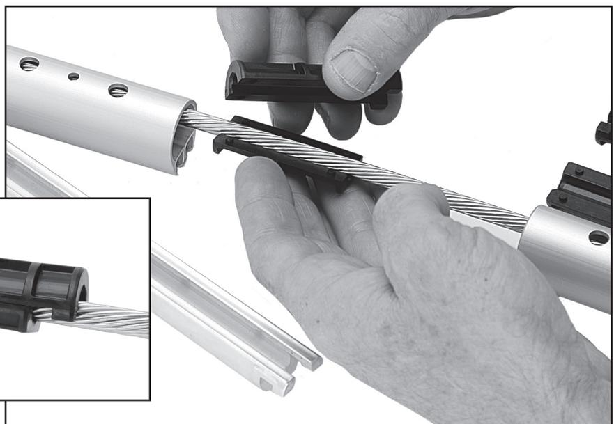
Slip connector on wire, mating hook of plastic bushing with connector.
