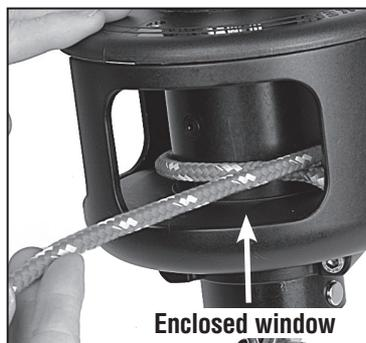
Run line through enclosed window in guard and into hole in bottom flange of spool. Tie a small overhand knot and pull it up under drum assembly.
