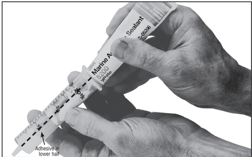
Start plunger into injector and immediately hold upright so plunger is down and applicator tip is up.
