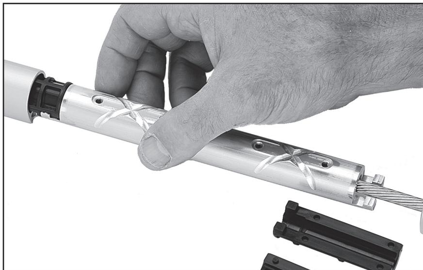
Put a drop of red Loctite® adhesive into screw holes.
