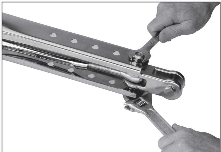
Check foil height at top; set and secure using hex key.
