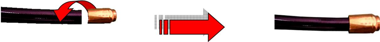
2. Insert the steel tapered end-piece into the stainless steel nut, and tighten very firmly on the male tapered union.
