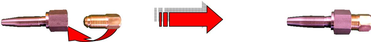
3. Lightly grease the tip of the stainless steel cone and screw it straight into the brass union. Stop where the steel threading disappears into the brass end-piece (a gap of approximately 7mm between the nut and the brass union)
