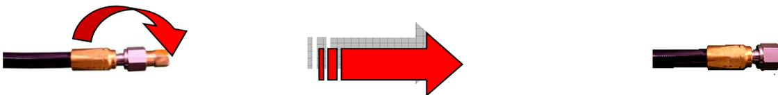
5. **IMPORTANT:** Check carefully that the end-piece does not block the hose:
